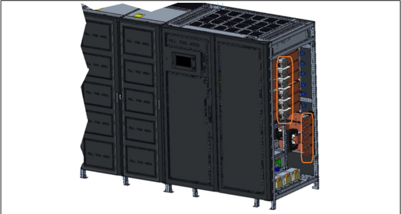
Figure 3.48 Front View, Mains and Bypass Copper Busbars Connections from AC Cabinet to the STS
