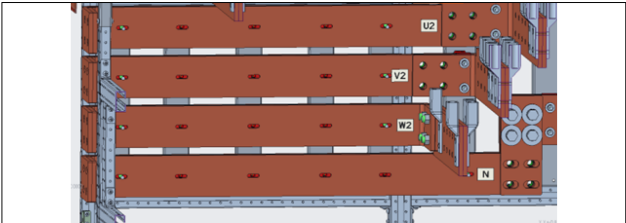
Figure 3.47 Front View, Mains and Bypass Copper Busbars Connections from AC Cabinet to the STS
