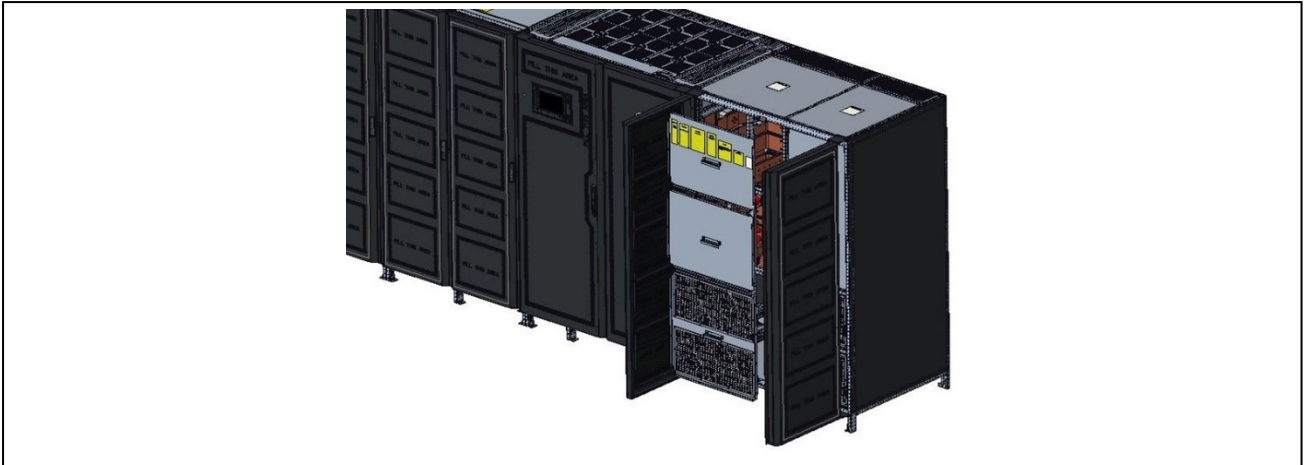
Figure 3.39 Removing AC Cabinet Second Access Panels
