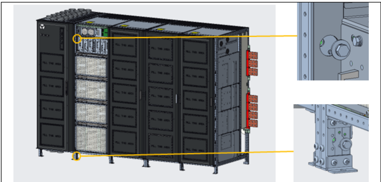
Figure 3.19 Front View, Mechanically Securing the DC Cabinet to the Core Cubicle
