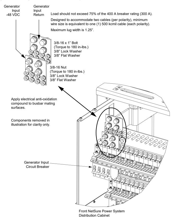
Figure 12.3 Vertiv™ NetSure™ 7100 (582127000203 or 582127000503) Installed in WIC
