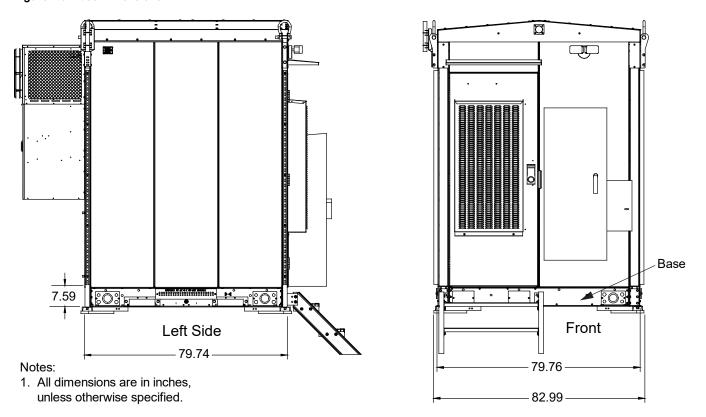
Figure 2.7 Conduit Knockout Locations in WIC Base Pan
