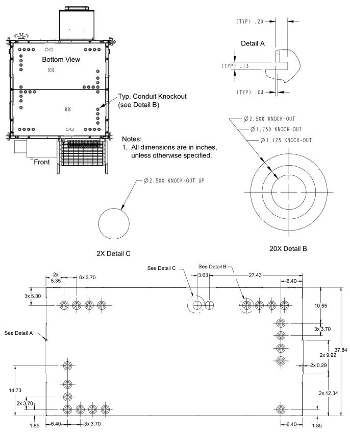
Bottom Cover Panel Conduit Knockout Locations and Dimensions
