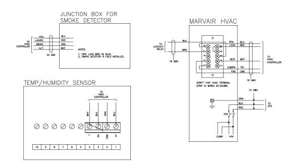
Figure 16.1 F2018009 Direct Air Cooling (DAC) and HVAC Schematic Diagram (cont'd from previous page)
