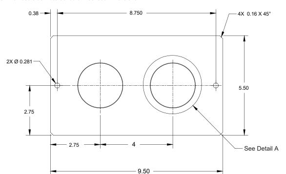
Figure 2.8 WIC Base Side Plate Conduit Knockout Dimensions
