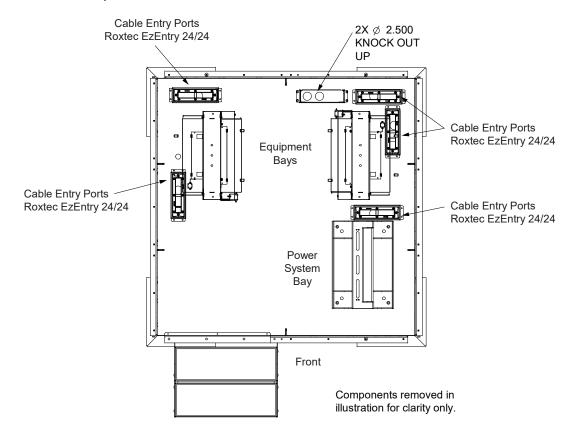
Figure 2.17 Wall Cable Entry Ports
