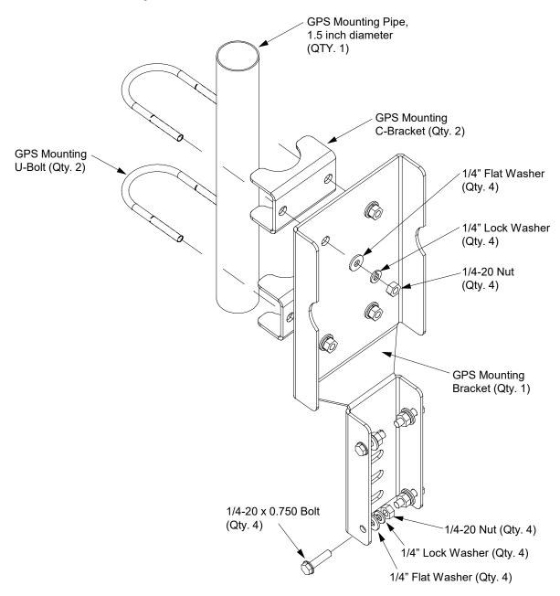
Figure 7.2 Installing the GPS Antennae Mounting Bracket Kit P/N 564693
