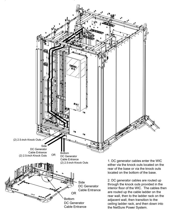
Figure 12.2 Connecting DC Generator Cable to Generator Input Circuit Breaker Kit P/N 564219
