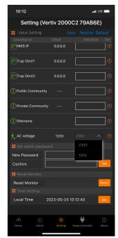
V1.00.18 and Later Versions (such as V1.10.03) Showing 120V or 230V AC Input Voltage Selection, Default at 230V, Selectable to 120V
