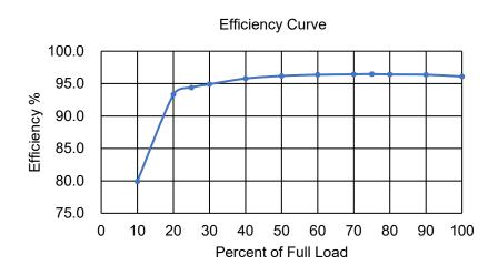
Figure 1.5 Efficiency Curve (@ 220 VAC, 60 Hz)
