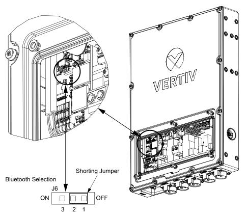
Bluetooth ON: Shorting jumper is installed between terminals 2 and 3 of J6.
