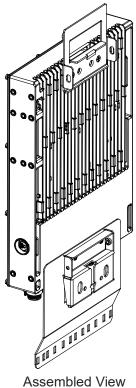
Mounting to a pole shown. Wall mounting similar. Flag Mounting Flat Mounting Previously Previously Mounted Mounted Bracket Bracket M6x16 Hex Head Screw (with lock washer and flat washer) Torque to 66 in-lbs.
