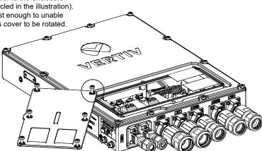
3. Rotate the access cover around the screw shown circled in the illustration.
