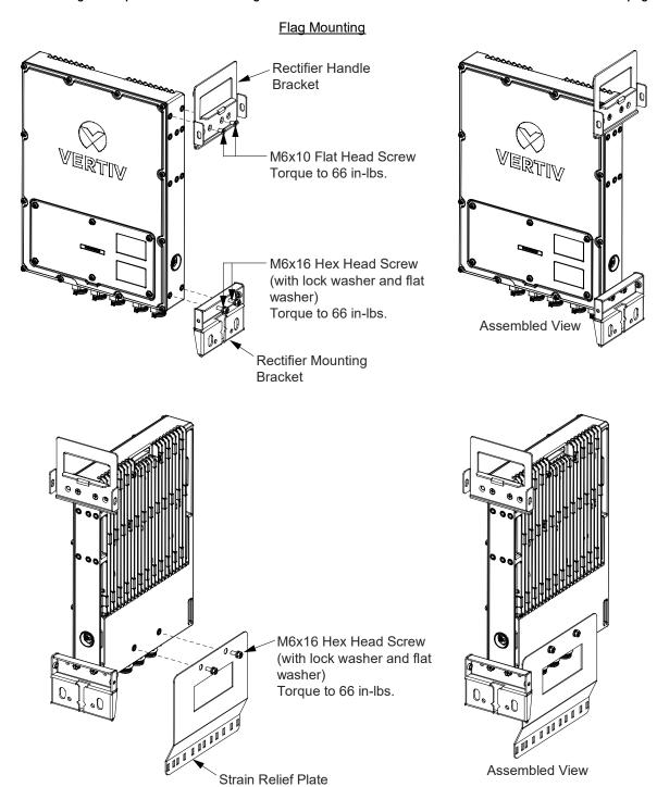
Figure 3.4 Installing the Top and Bottom Mounting Brackets and Strain Relief Plate to the Rectifier (cont'd from previous page)
