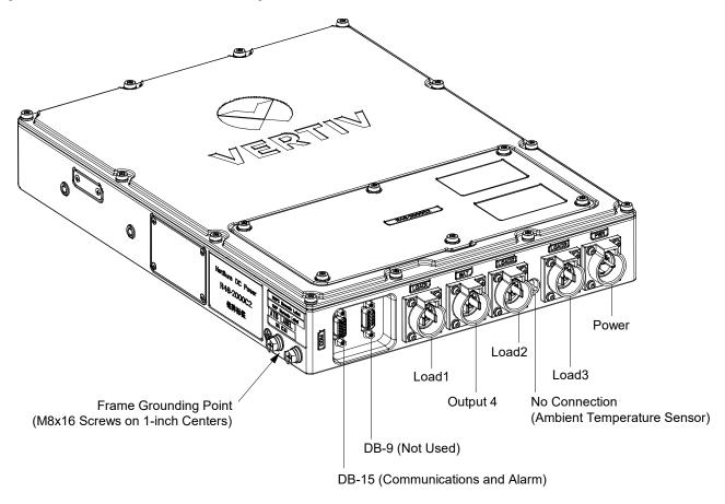
**Figure 4.1 Rectifier Ground Connection**
