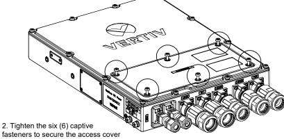
fasteners to secure the access cover to the enclosure (shown circled in the illustration). Torque to 22 in-lbs.
