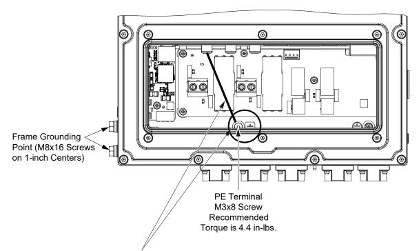
IMPORTANT: Rectifier is factory +RTN bonded to chassis. When chassis is bonded to earth ring ground, then +RTN will also be referenced to Earth. This means rectifier will be a DEFAULT -48 VDC power system. Internal +RTN wire is factory connected to the PE terminal M3 screw shown above, next to the earth symbol. If customer chooses to float DC bus, access panel must be opened, and this wire must be unterminated and insulated.
