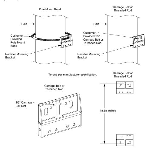
Figure 3.4 Installing the Top and Bottom Mounting Brackets and Strain Relief Plate to the Rectifier (cont'd on next page)
