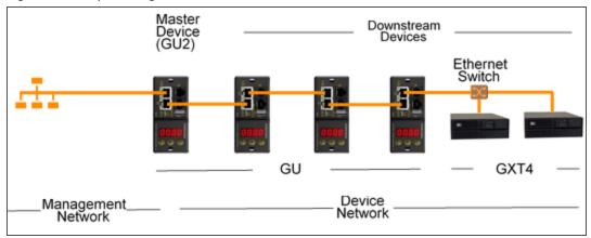
The IMD-3E is the default intelligence card for Vertiv™Geist™ GU2 rPDUs, which include switched (model numbers beginning with MNS), outlet monitored (model numbers beginning with MNR) and switched plus outlet monitored (model numbers beginning with MNU) products. To serve as the Master rPDU, rPDUs with a legacy intelligence card must first be upgraded to the IMD-3E.
