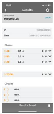
NOTE: The unit serial number is displayed in the title bar of the Readings screen. This serial number matches the serial number displayed on the label of the rPDU.
