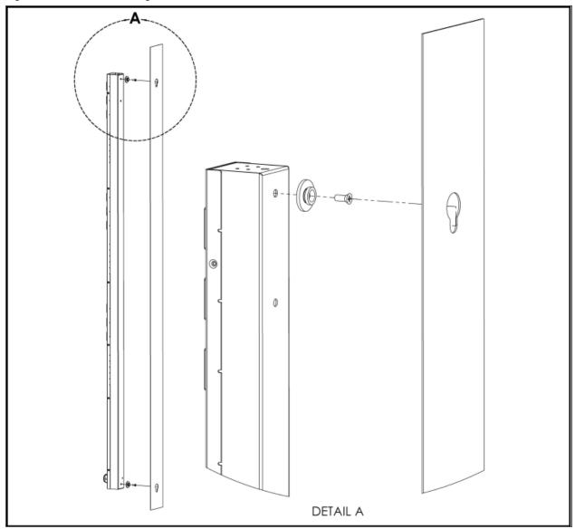
Figure 2.5 Toolless Full-Length Brackets
