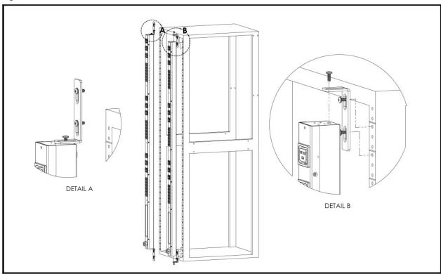
Figure 2.3 Vertical Extension Brackets
