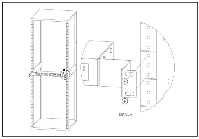
Figure 2.13 19" Horizontal/Panel-Mount Brackets
