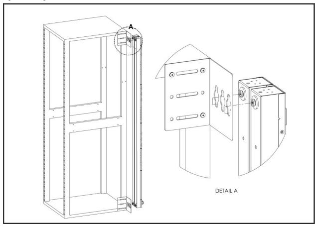
Figure 2.7 Offset/Side-Mount Brackets
