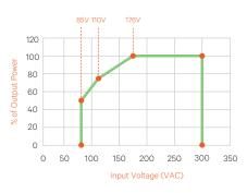
Figure 1: Output Power vs. Input Voltage and Vo > 48V at Temp < 55°C
