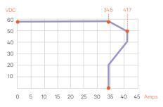
Figure 2: Output Voltage vs. Output Current at Maximum Output Power 2000 W
