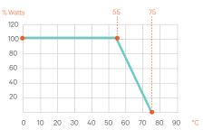
Figure 3: Output Power vs. Temperature at 290 VAC ≥ Vin ≥ 200 VAC
