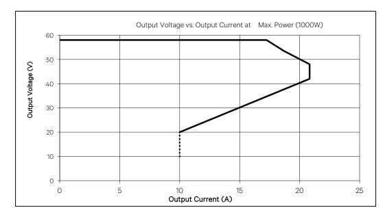
Figure 1.1 Output Voltage vs. Output Current with AC /DC input
