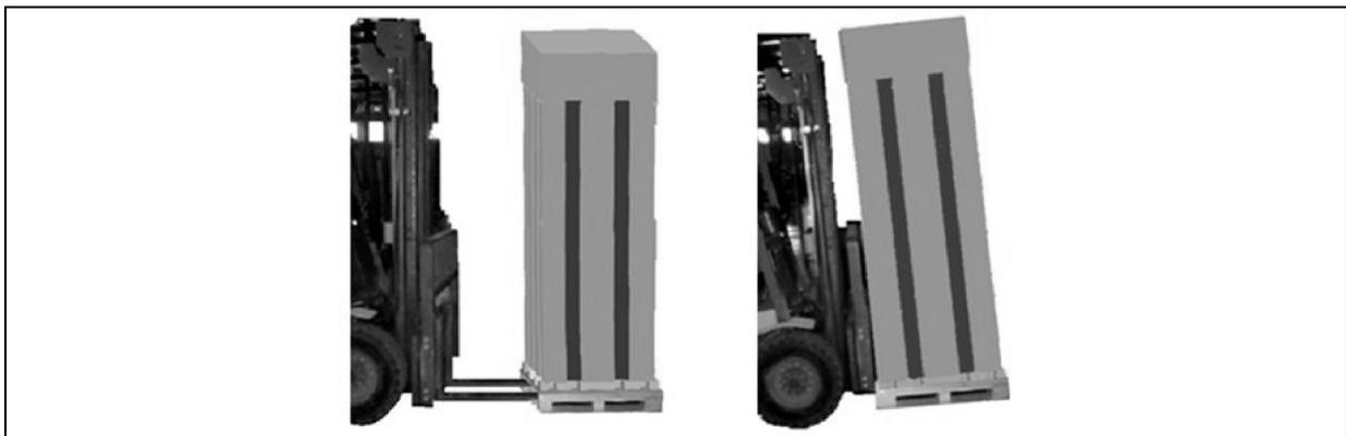
When moving the packaged unit, align the fork arms with the unit center of gravity and do not tilt the unit more than 20 degrees in any direction to prevent the unit from falling over.
