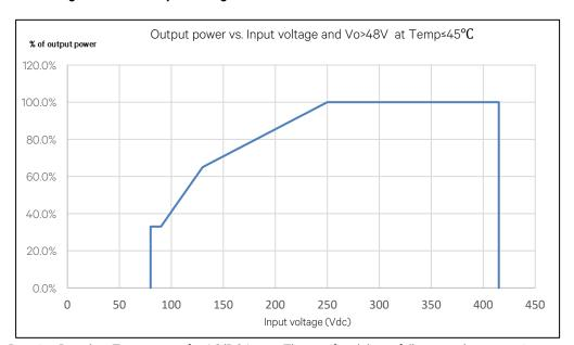
Figure 1.5 Power Derating Based on DC Input Voltage
