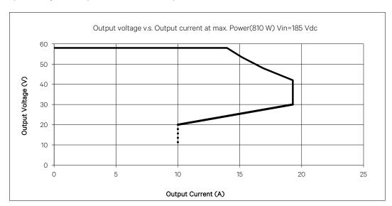
Figure 1.3 Output Voltage vs. Output Current with DC input(810W)
