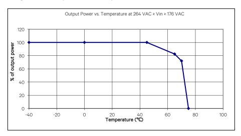
Figure 1.6 Power Derating Based on Temperature for AC Input
