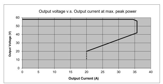
Figure 1.2: Output Voltage vs. Output Current at Maximum Peak Power 2000W
