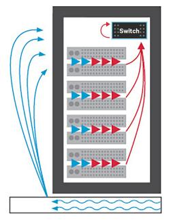
Network switches mounted at the top and rear of the rack are susceptible to heated air from the servers. This hot air is recirculated, putting stress on the device.
