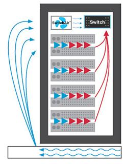
Vertiv<sup>™</sup> Geist<sup>™</sup> SwitchAir<sup>™</sup> products direct cool air to the network switches, significantly lowering operating temperatures.
