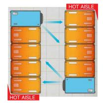
Liebert CRV systems operating in hot aisle/cold aisle configuration.
