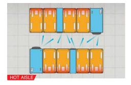
As rack densities increase, inserting additional cooling units within the row will meet cooling demand.
