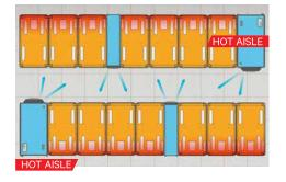
By placing Liebert CRV 600mm units at either end of the rows and inserting 300mm wide units throughout, the Liebert iCOM<sup>™</sup> controls ensure that the aisle is evenly pressurized, simulating cold aisle containment.
