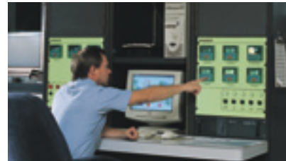
Our state-of-the-art psychrometric laboratory allows us to test units under a wide variety of temperature and humidity conditions.
