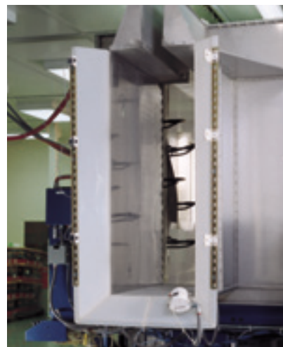
Powder coated exterior panels — Solvent-free process provides a durable, high quality, scratch-resistant finish.
