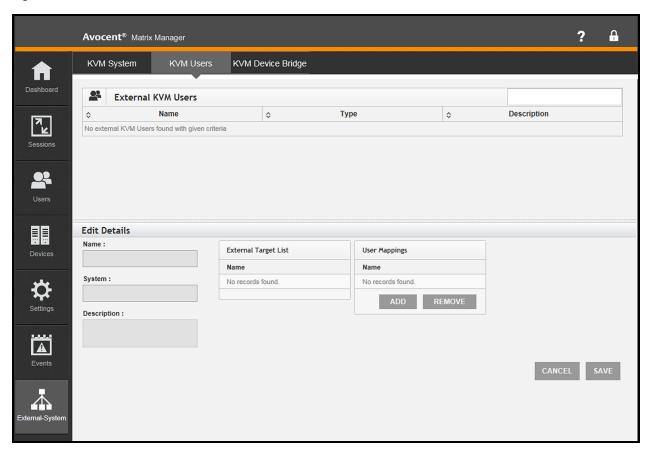
The Edit Details section of the external KVM Users screen can be used to view the external username, corresponding external system and the list of external targets/transmitters which the user can access.
