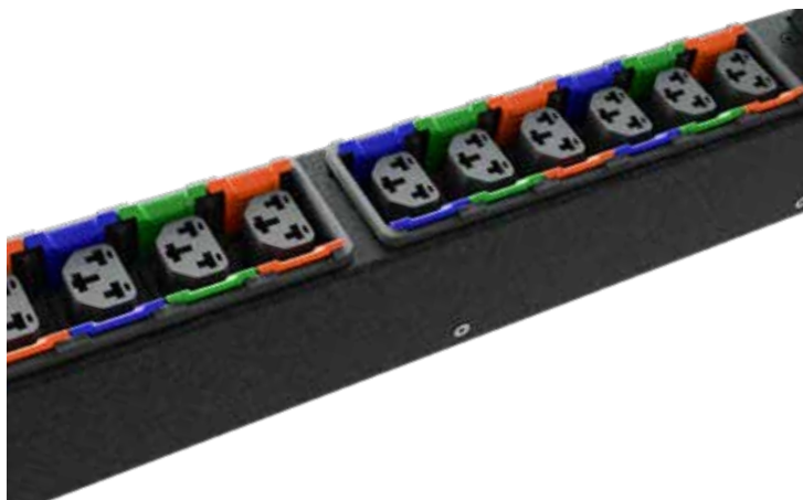
Receptacles on the Vertiv Geist rPDUs are color coded by phase to simplify load balancing.
