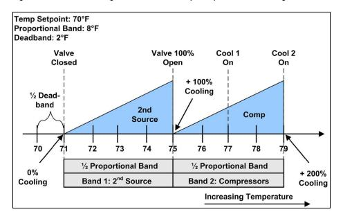
Figure 3.17 Second Cooling Source and Two-Step Compressorized Cooling
