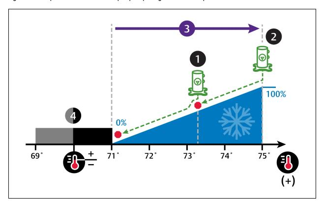
Figure 3.5 Compressor Control—Two Step Capacity Using One Scroll Compressor with Unloaders
