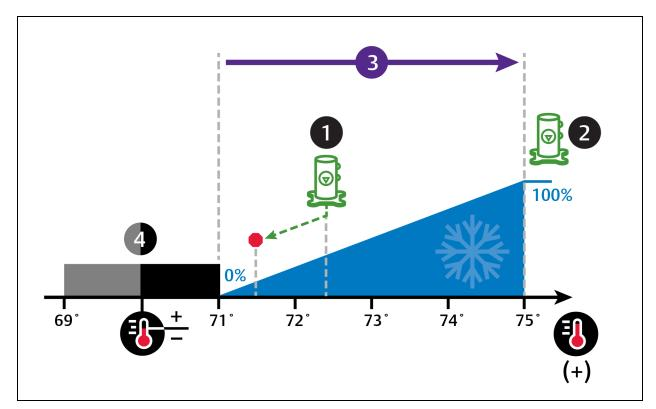
Figure 3.8 Compressor Control—Single Digital Scroll Compressor
