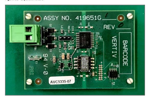
NOTE: The TB1 for RS-485 Terminal Block is used if a Sitelink/Sitescan connection and MODBUS or BACnet MSTP is required simultaneously.
