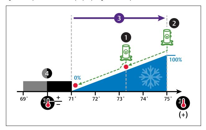
Figure 3.4 Compressor Control—Two Step Capacity Using Two Scroll Compressors without Unloaders
