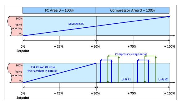
Figure 3.18 Freecooling and Compressorized Operation
