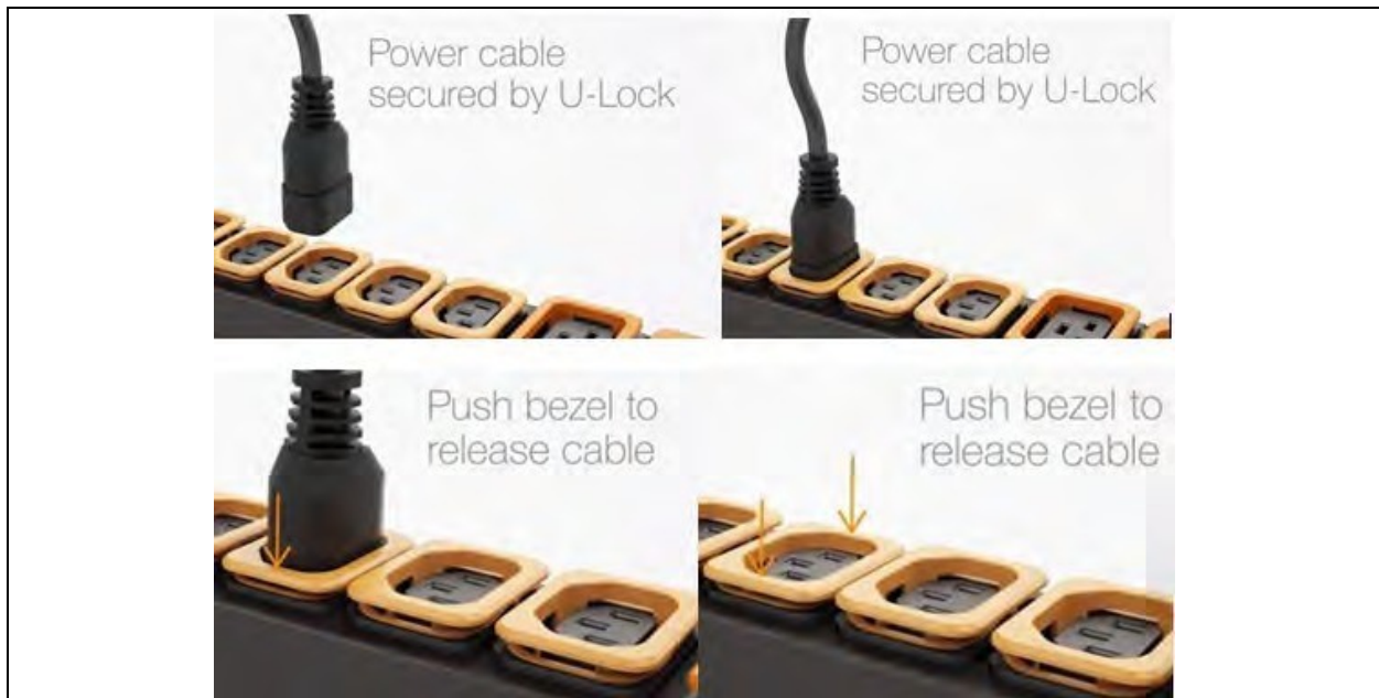
Figure 3.3 U-Lock Cord Retention Operation
