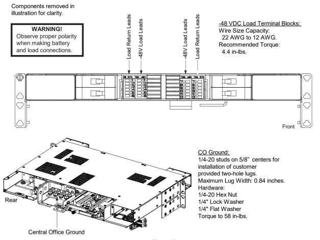
Figure 13 Load Distribution Wiring, Input Battery Wiring, and CO Ground Wiring (Lists BA and NA)
