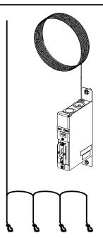
Yellow Jumper/Alarm Lead (P/N 524384) (for use when more than one Battery Disconnect Units are ordered)
