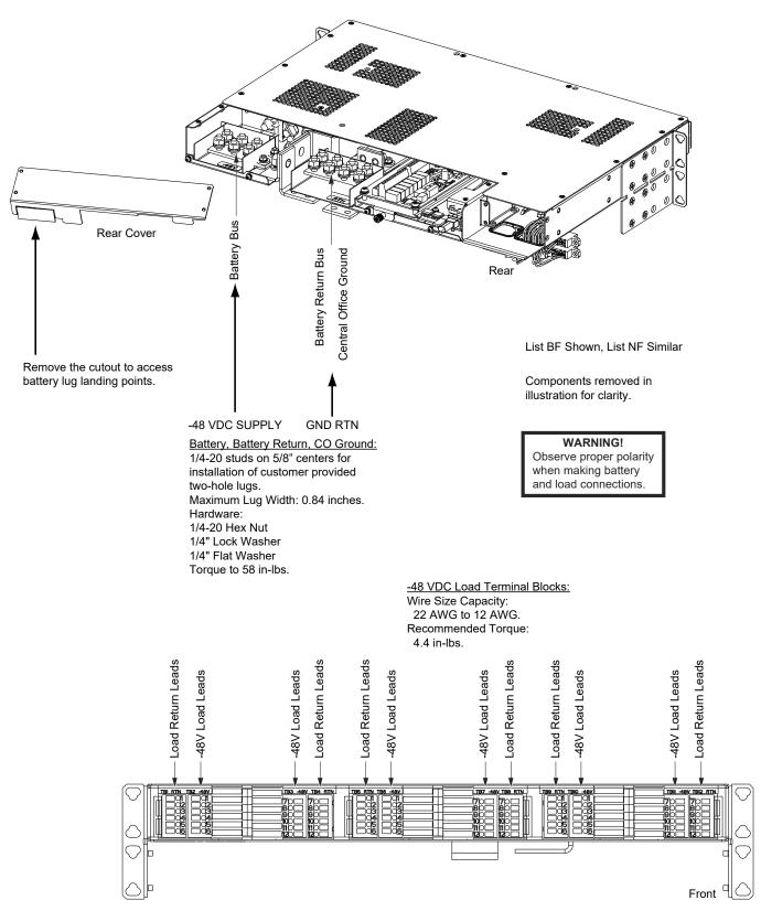
Figure 11 Load Distribution Wiring, Input Battery Wiring, and CO Ground Wiring (Lists BF and NF)
