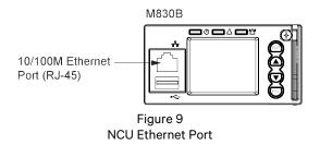
Note: If your system has an IB4 board, DO NOT connect your Local Area Network (LAN) to the NCU front Ethernet port.
