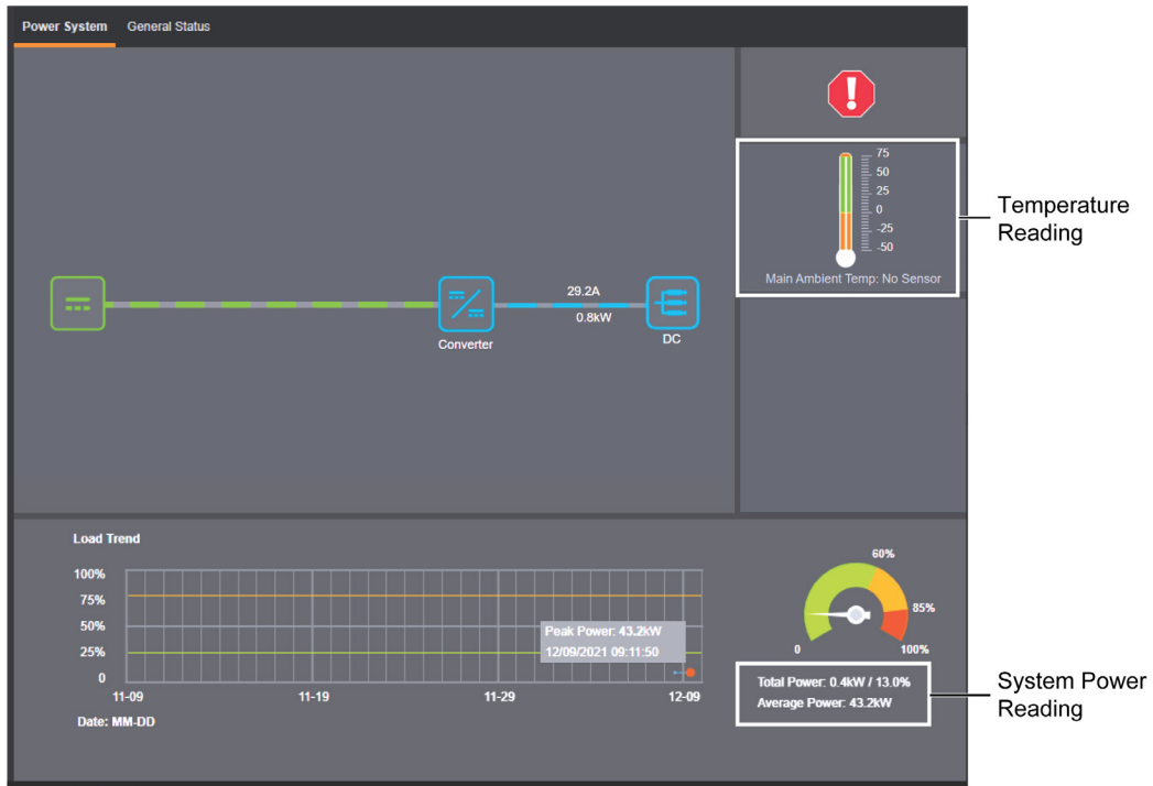
Figure 9-9 Power System Status Tab
