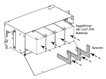
3. Connect all four EaglePicher batteries using wires (Part Number 541424) crimped with 12-10 AWG Faston receptacle on each end, as shown in **Figure 18**.
