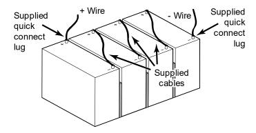
4. Attach the cabinet wires to + and - terminals. Refer to Figure 10.
