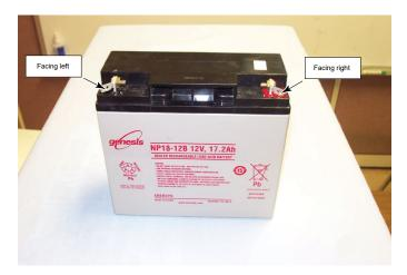
4. Attach a fast-on lug to the negative and positive terminal of the second battery facing left and one of the fast-on lugged cables to the positive terminal off the battery. Repeat for third and fourth batteries in the string. See **Figure 23**.
