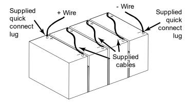
4. Attach the cabinet wires to + and - terminals. Refer to Figure 13.
