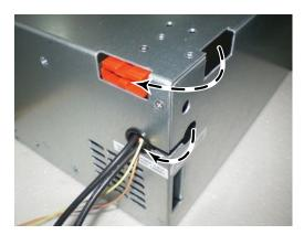
3. Install the frame ground landing point adapter P/N 556872 to the left or right side of the battery cabinet, as shown in **Figure 5**.
