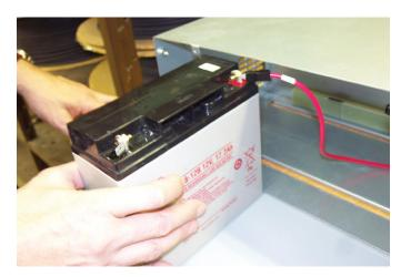
6. Place inner battery spacer next to battery. Make sure that the positive long lead cable is resting on the rear spacer. See **Figure 25**.
