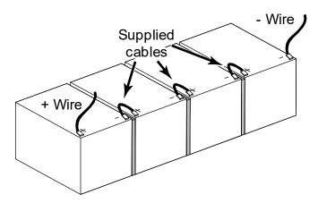
4. Attach the cabinet wires to + and - terminals. Refer to Figure 16.
