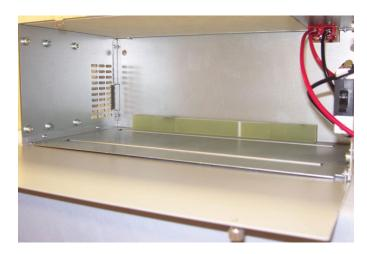
2. Take the (3) Inner Battery Spacers and break off the end portion of the spacer where indicated, as shown in **Figure 21**.
