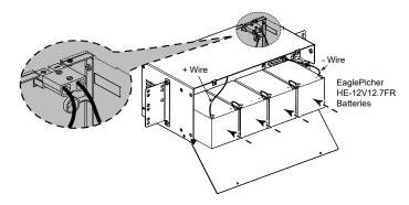
5. Refer to "Securing the Batteries Using the Strap" on page 25 for instructions on securing the batteries using the buckle strap that is bundled along with the cabinet.
