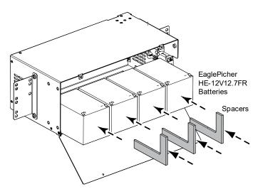
3. Connect all four EaglePicher batteries using supplied wires (Part Number 541424) crimped with 12-10 AWG Faston receptacle on each end, as shown in **Figure 15**.
