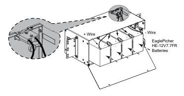
5. Refer to "Securing the Batteries Using the Strap" on page 25 for instructions on securing the batteries using the buckle strap that is bundled along with the cabinet.
