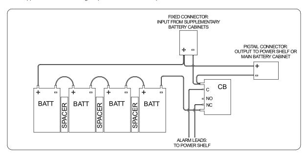
Figure 32: Typical Internal Wiring Layout - 582136600 System
