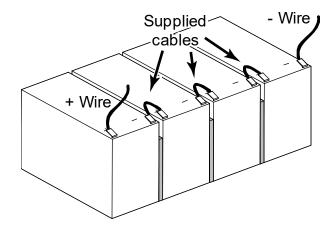
4. Attach the cabinet wires to + and - terminals. Refer to Figure 19.
