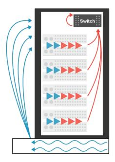
Network switches mounted at the top and rear of the rack are susceptible to heated air from the servers. This hot air is recirculated, putting stress on the device.
