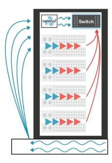
SwitchAir™ products direct cool air to the network switches, significantly lowering operating temperatures.
