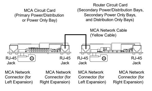
Figure 1.8 Removing Cables – Detail MCA-B
