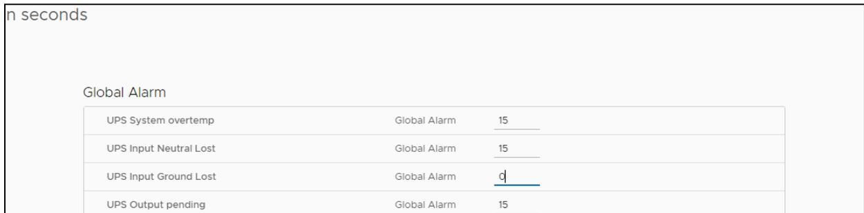
As shown in **Figure 3.42** above , the delay time of the UPS Input Ground Lost alarm is modified to 0 seconds. It indicates that the alarm will trigger immediately and the warning rule will be executed.
