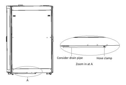
Figure 2-4 Schematic diagram of down pipe drainage
