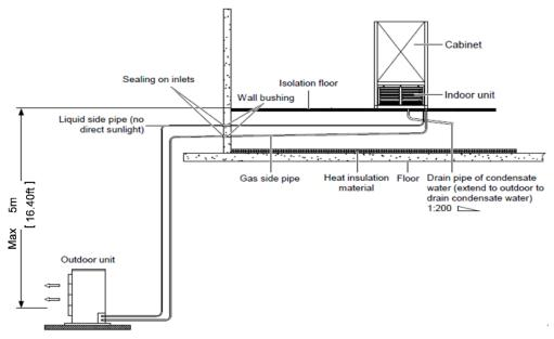
Figure 2-2 The Condensing unit is installed lower than the indoor unit
