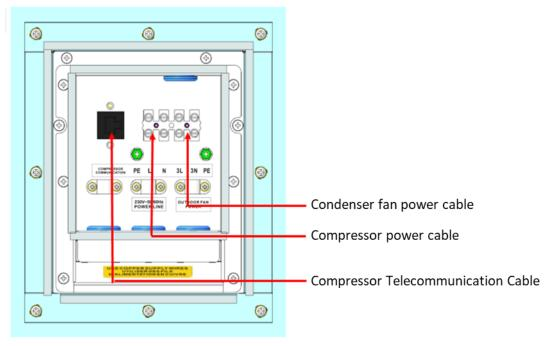
Figure 3-2 Condensing unit cable connection
