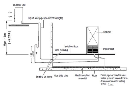
Figure 2-1 The Condensing unit is installed higher than the indoor unit
