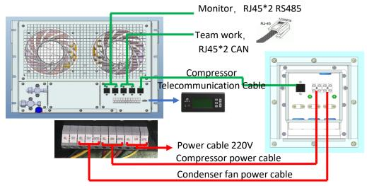
Figure 3-3 Overview of the cabling connections
