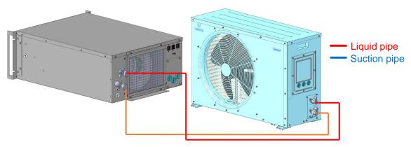
Figure 2-4 Schematic diagram of pipeline connection
