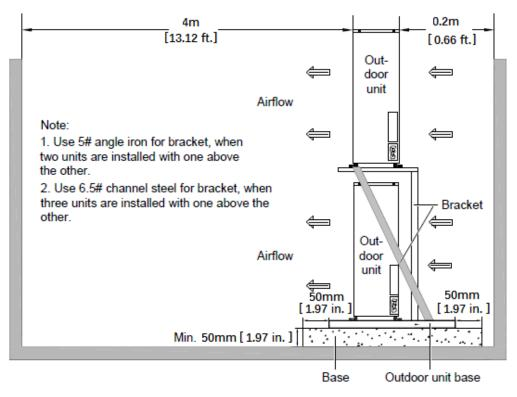
Figure 2-3 Installing multiple condensing units one above the other
