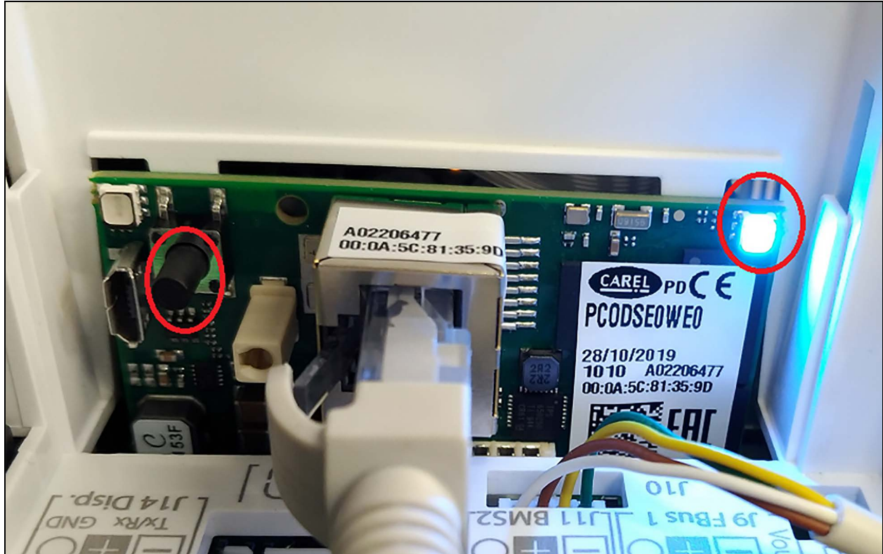
Figure 4.20 Black Button and LED Light
