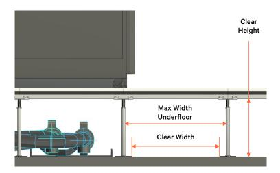
This illustration depicts the clearance required to accommodate underground piping in a facility with a raised-floor design. Dimensions will vary from site to site.
