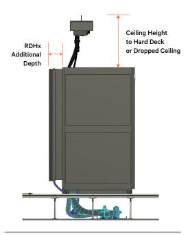
This illustration shows how running a rear-door heat exchanger adds depth to racks.
