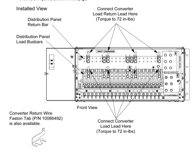
Figure 9: Connecting Converter Load Return Cables to the Return Bar with the Converter Return Wire Faston Tab and
