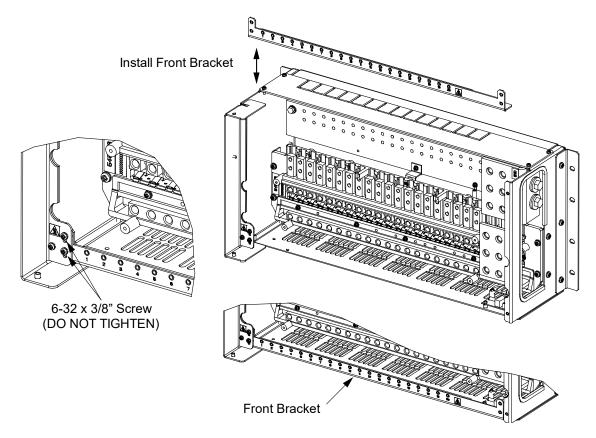
[ ] 6. Orient the kit supplied right side mounting bracket as shown in **Figure 4**. Secure the right side mounting bracket to the distribution panel with kit supplied hardware as shown in **Figure 4**. Torque hardware as indicated in **Figure 4**. Secure the front mounting bracket to the right side mounting bracket as shown in **Figure 4**. DO NOT TIGHTEN HARDWARE (hardware will be tightened during converter installation).
