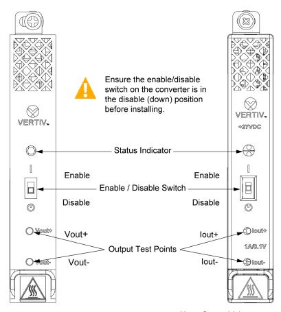
Note: Output Voltage measurement on the +27 VDC Vertiv™ eSure™ Bullet Converter represents output current. 1A/0.1V
