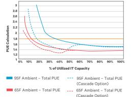
\*CRV inlet air temperature 75° F. PUE is a measure of how efficiently a computer data center uses its power; specifically, how much of the power is actually used by the computing equipment (in contrast to cooling and other overhead).
