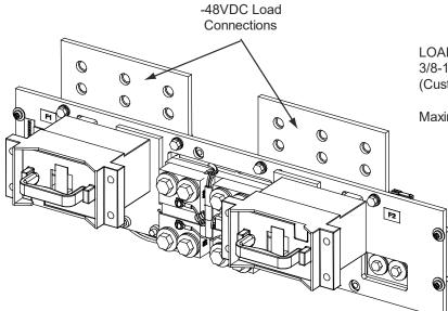
LOAD CONNECTIONS 3/8-16 Captive Nuts on 1" Centers (Customer must supply or order additional hardware)
