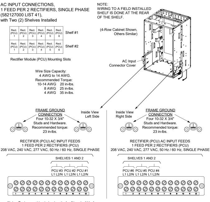
Note: Customer wiring to top terminals of terminal blocks. For fewer power shelves than shown, only the connections for the installed shelves are present.
