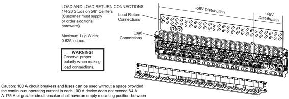
A 175 A or greater circuit breaker shall have an empty mounting position between it and any other overcurrent protective device.
