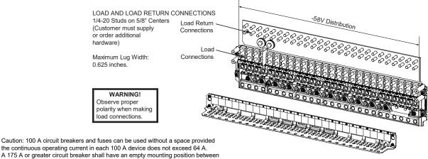
A 175 A or greater circuit breaker shall have an empty mounting position between it and any other overcurrent protective device.
