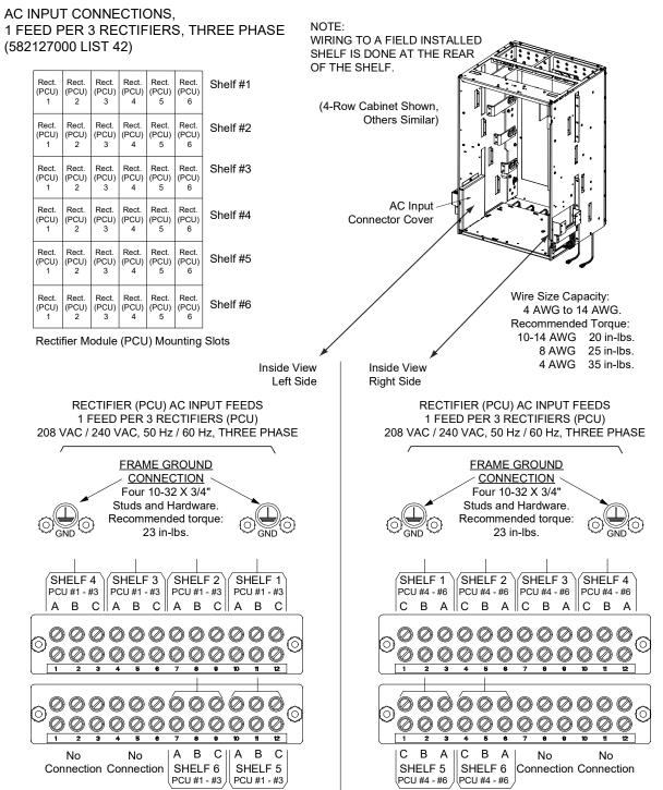
Note: Customer wiring to top terminals of terminal blocks.
