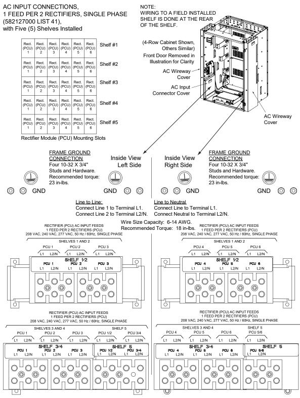
AC Input Connections to AC Input Termination Assembly List 41 Illustration when used with 588705300 (Nominal 208 VAC, 240 VAC) or 588705400 (Nominal 208 VAC, 240 VAC, 277 VAC) Module Mounting Assemblies with Rectifiers (1 Feed per 2 Rectifiers, Single Phase) - with Four (4) Shelves Installed
