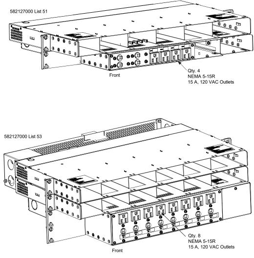
Figure 9 AC Output Connections (List 51, List 53)
