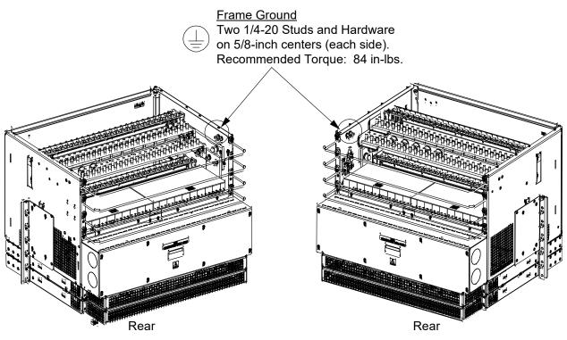
Figure 2 List 600, 601, 900, 901 Power System Shelf Frame Ground Connection
