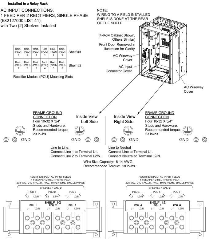
AC Input Connections to AC Input Termination Assembly List 41 Illustration when used with 588705300 (Nominal 208 VAC, 240 VAC) or 588705400 (Nominal 208 VAC, 240 VAC, 277 VAC) Module Mounting Assemblies with Rectifiers (1 Feed per 2 Rectifiers, Single Phase) - with One (1) Shelf Installed
