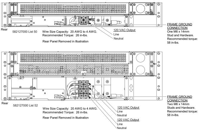
Figure 8 AC Output Connections (List 50, List 52)
