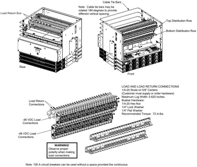
current in each 100 A device does not exceed 64 A. A 175 A or greater circuit breaker SHALL HAVE an empty mounting position between it and any other overcurrent protective device.
