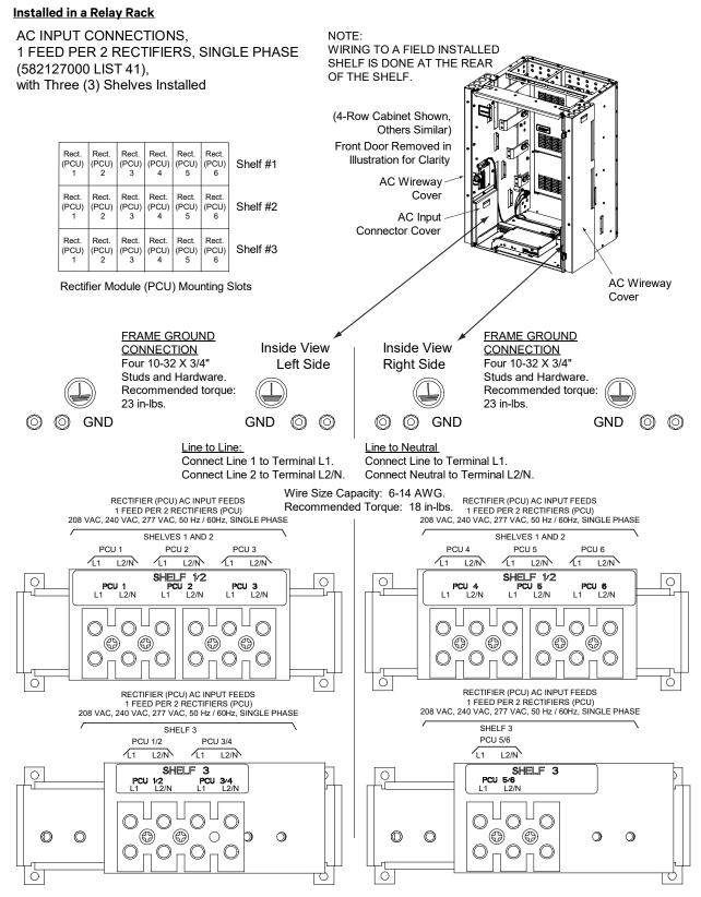
AC Input Connections to AC Input Termination Assembly List 41 Illustration when used with 588705300 (Nominal 208 VAC, 240 VAC) or 588705400 (Nominal 208 VAC, 240 VAC, 277 VAC) Module Mounting Assemblies with Rectifiers (1 Feed per 2 Rectifiers, Single Phase) - with Two (2) Shelves Installed
