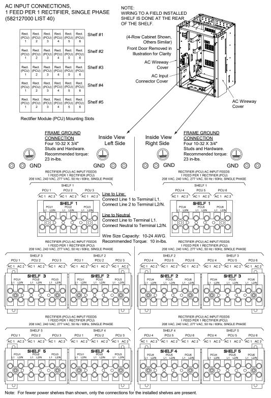
AC Input Connections to AC Input Termination Assembly List 41 Illustration when used with 588705300 (Nominal 208 VAC, 240 VAC) or 588705400 (Nominal 208 VAC, 240 VAC, 277 VAC) Module Mounting Assemblies with Rectifiers (1 Feed per 2 Rectifiers, Single Phase) - with Five (5) Shelves Installed
