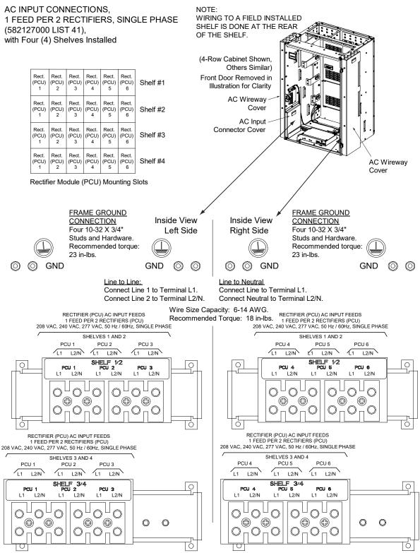
AC Input Connections to AC Input Termination Assembly List 41 Illustration when used with 588705300 (Nominal 208 VAC, 240 VAC) or 588705400 (Nominal 208 VAC, 240 VAC, 277 VAC) Module Mounting Assemblies with Rectifiers (1 Feed per 2 Rectifiers, Single Phase) - with Three (3) Shelves Installed
