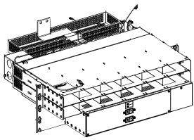
Maximum system output power when equipped with two (2) 23-inch-wide inverter shelf is 12kVA at 40  $^{\circ}$ C and 6kVA at 65  $^{\circ}$ C.
