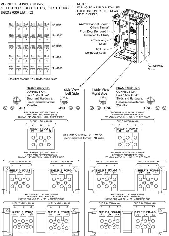
Note: For fewer power shelves than shown, only the connections for the installed shelves are present. Note: The three-phase input is internally distributed within the system to provide a single-phase line to line connection to each rectifier position, evenly distributed across the three phases.
