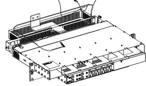
Maximum system output power when equipped with one (1) 23-inch-wide inverter shelf is 5.76kVA at 40 °C and 3kVA at 65 °C.
