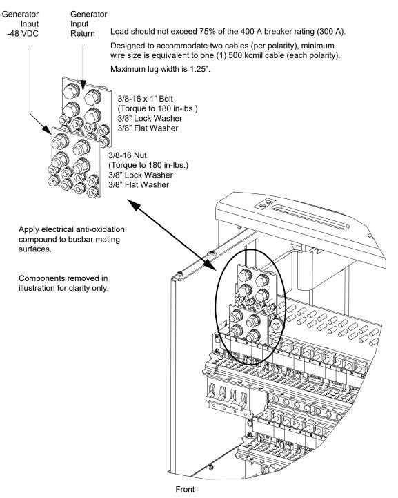
Figure 1 Wiring Input Generator Kit P/N 564219
