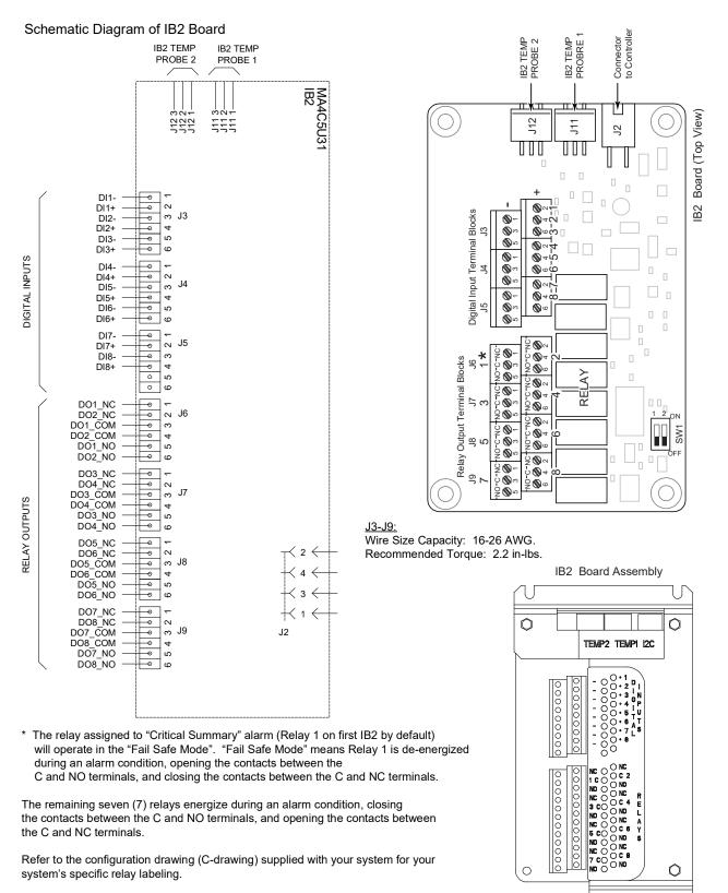
Not all I/O points are available for customer connection (some are used for factory system connections).
