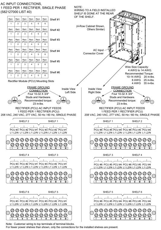
Line to Line: Connect Line 1 to Terminal L1. Connect Line 2 to Terminal L2/N.
