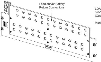
LOAD AND/OR BATTERY RETURN CONNECTIONS 3/8-16 Captive Nuts on 1" Centers (Customer must supply or order additional hardware)
