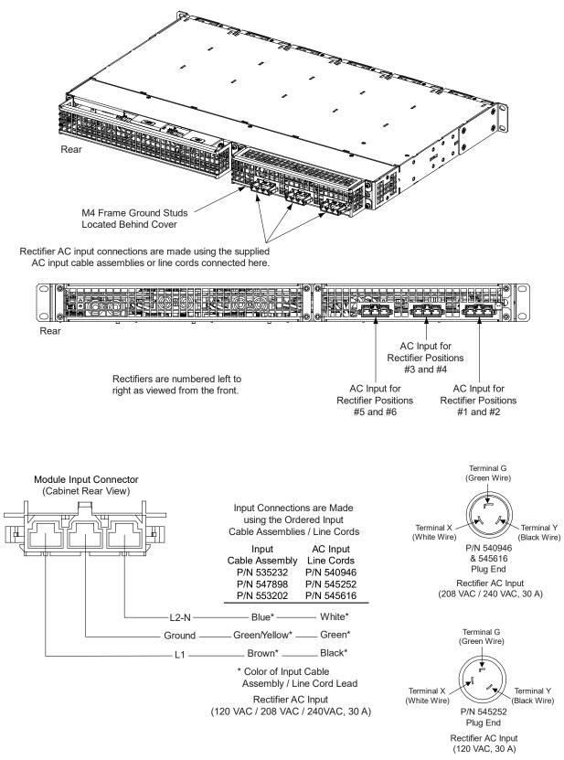
Figure 4 Input Connections, 588705300 List 03
