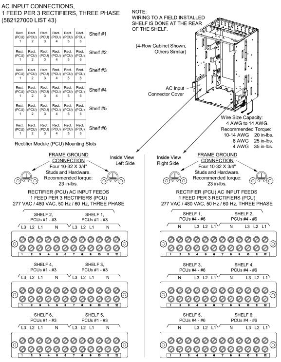
Note: Customer wiring to top terminals of terminal blocks.
