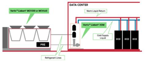
Working in tandem rear door Vertiv™ Liebert® DCD, the Vertiv™ Liebert® XDM integrates pumped refrigerant economization (PRE) to eliminate the need for chilled water, allowing you to easily and efficiently cool pods of high-density racks in your air-cooled data center.
