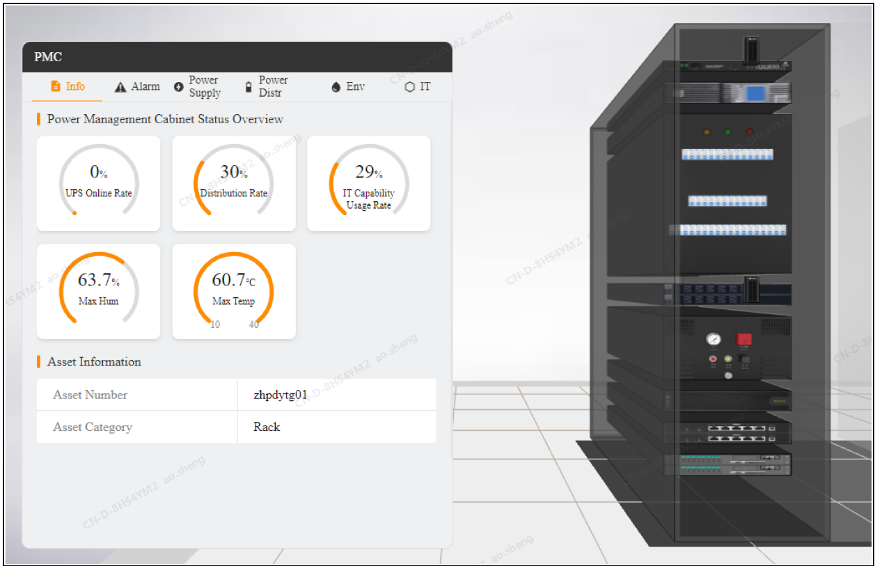
Figure 6.44 Single-Cabinet View of the PMC Cabinet at the Smart Row Site
