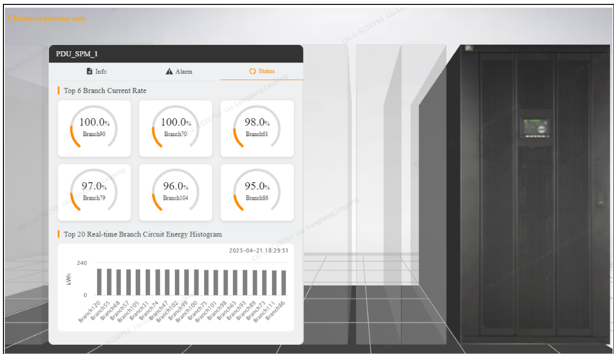
Figure 6.21 SPM Cabinet Status Card
