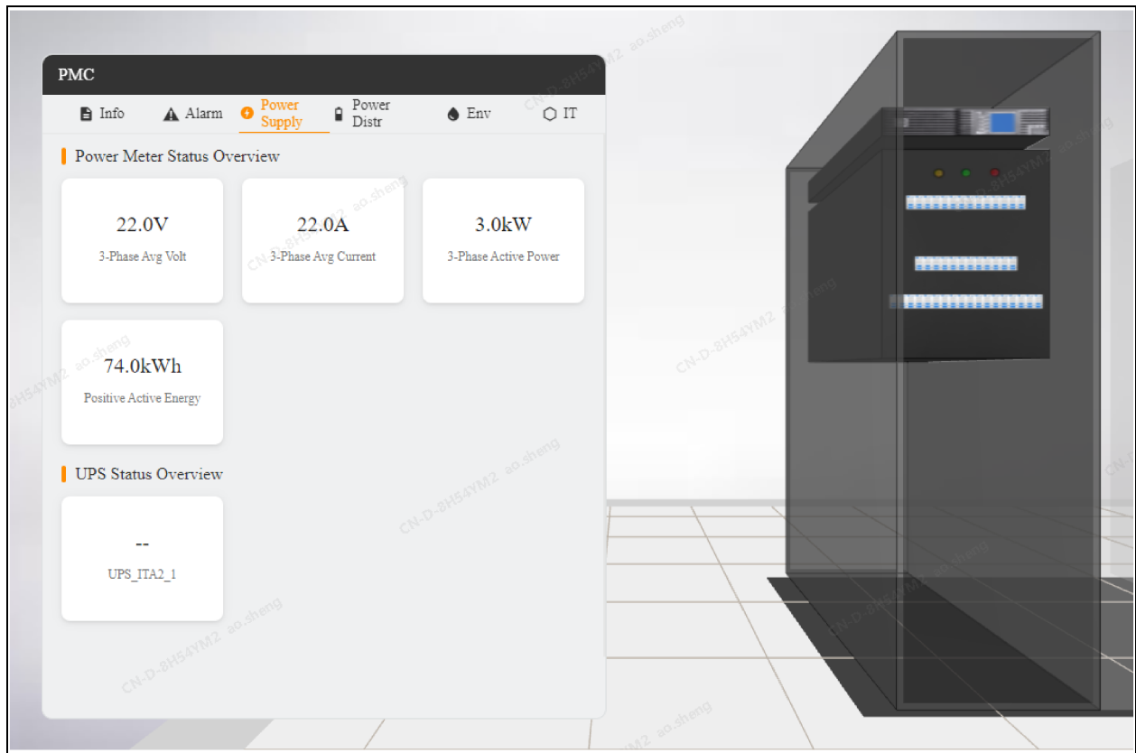
Figure 6.46 Power Supply Card of the PMC Cabinet is Displayed
