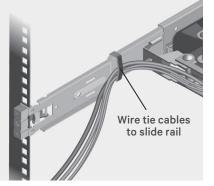
Secure the cables to the rear of the slide rail with a wire tie. Make sure the cables are not pulled too tight.
