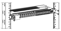
Figure 3-1 PDU48/300DF rack installation
