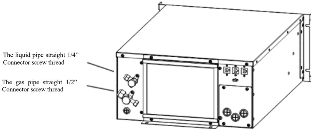
Figure 3-10 The pipe connection port
