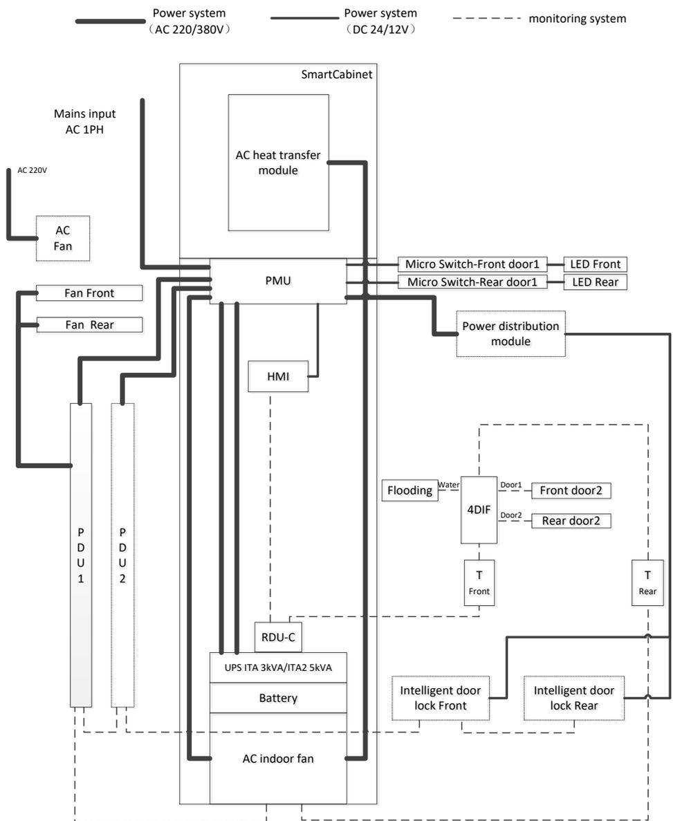
Figure 3-25 Total wiring diagram
