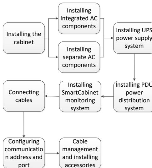
Figure 3-1 Flow chart of installation
