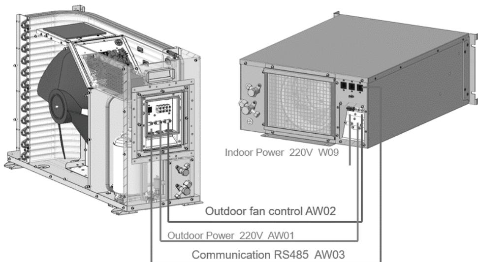
Figure 3-30 Connect the cables of indoor and outdoor unit
