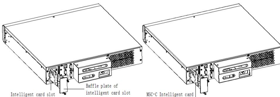
Figure 3-23 Schematic diagram of installing MSC intelligent monitoring card
