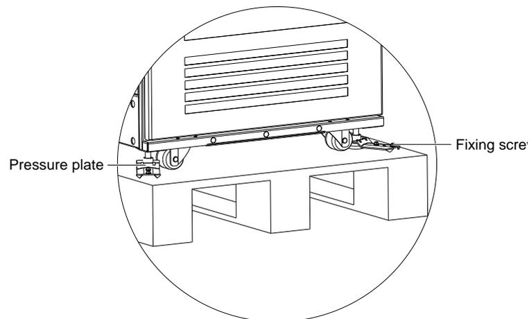
Figure 2-8 Removing the feet pressure plate
