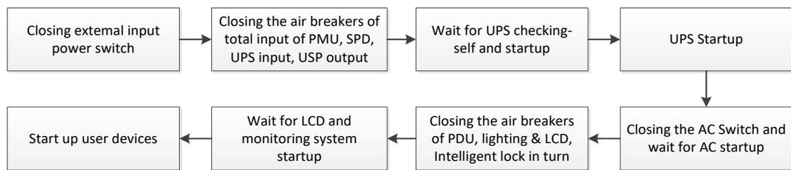
Figure 4-2 Startup flowchart
