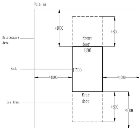
Figure 1-7 Space requirement of 800mm wide standard unit
