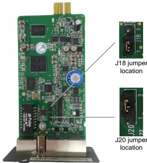
Figure 3-22 Jumper locations of the MSC intelligent monitoring card
