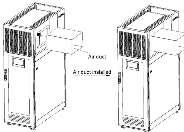
Figure 3-20 Installation of air duct
