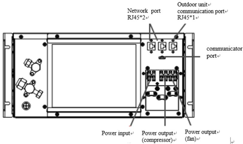
Figure 3-28 Connecting power cable of outdoor unit
