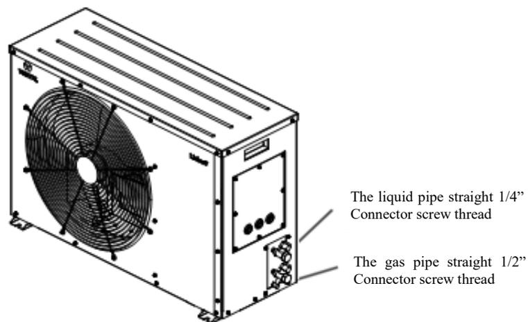
Figure 3-11 Outdoor refrigeration line interface
