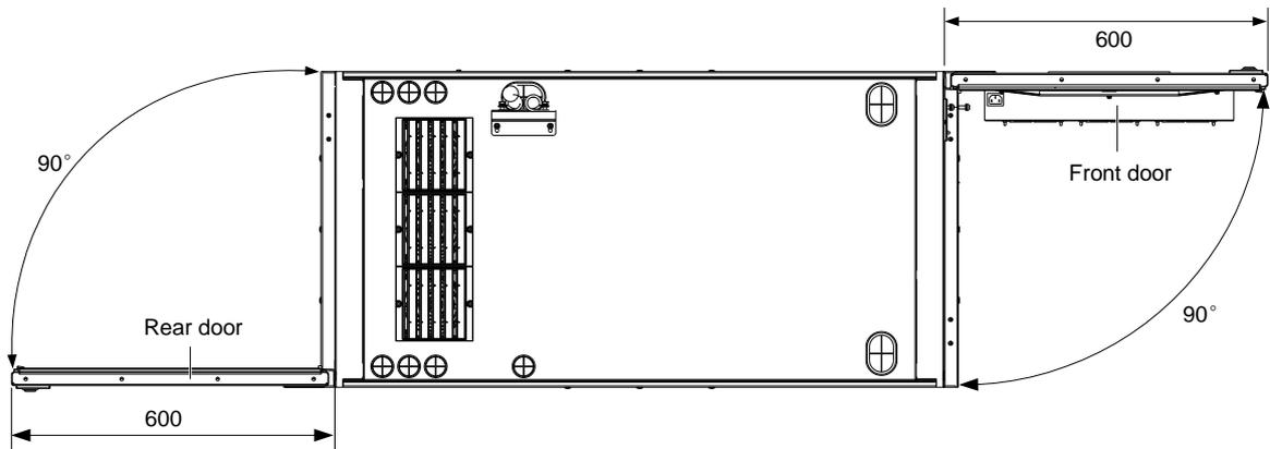
Figure 1-5 Required clearance for opening the front and rear door (Top view, unit: mm)
