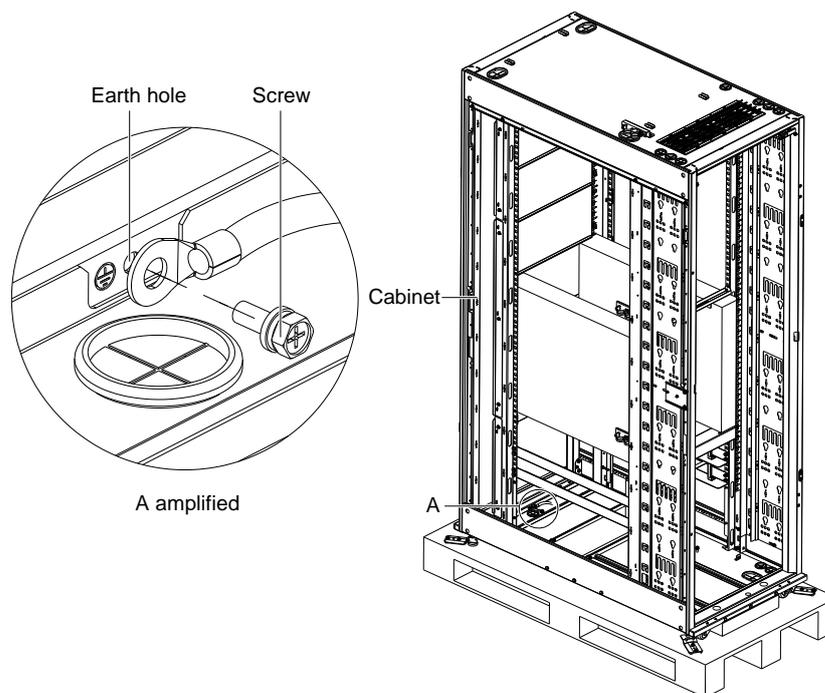
Figure 3-31 Connecting earth cable
