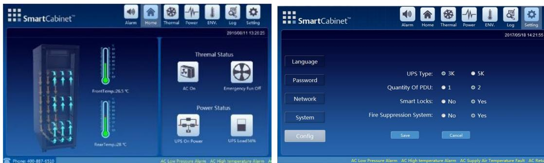
Figure 4-4 SmartCabinet LCD screen
