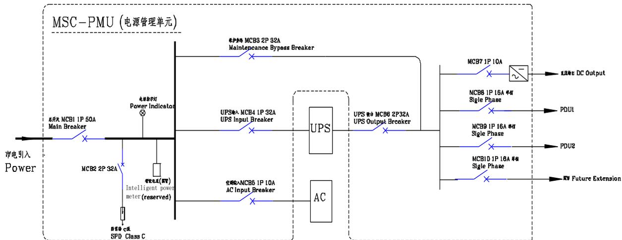
Figure 1 The schematic diagram of the SmartCabinet system distribution
