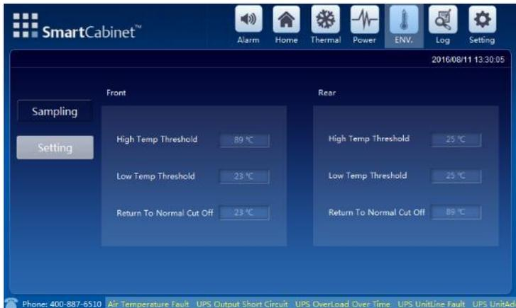
Figure 5-13 Environmental setting data screen(need a password to enter)
