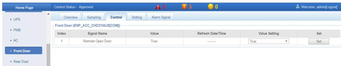
Figure 4-6 Remote door-opening control
