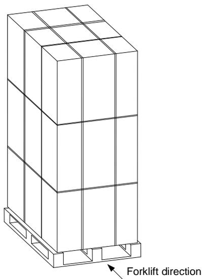
Figure 2-6 Forklift direction
