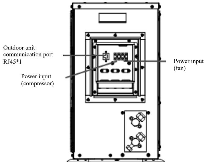
Figure 3-29 Connecting power cable of outdoor unit
