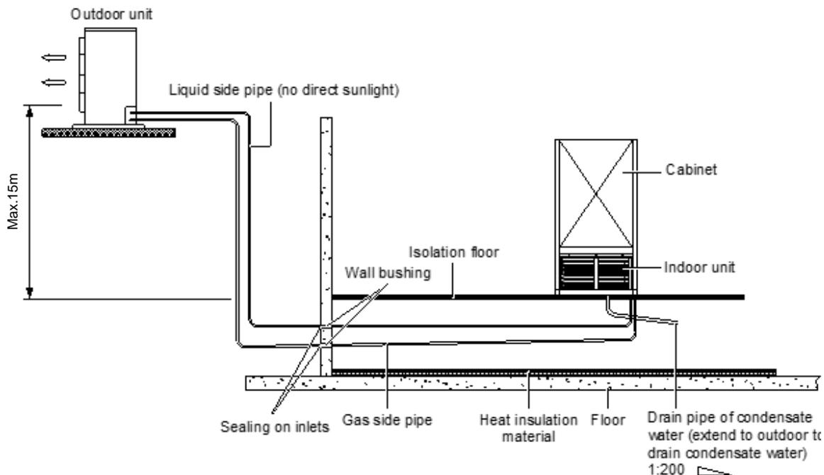
Figure 3-5 Outdoor unit installed higher than indoor unit
