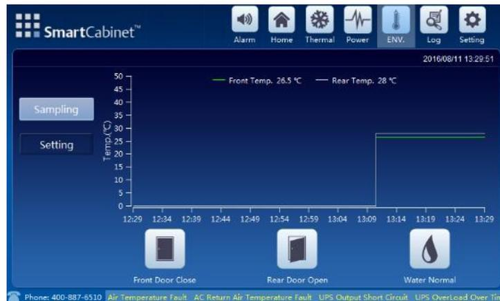
Figure 5-11 Environmental acquisition data screen
