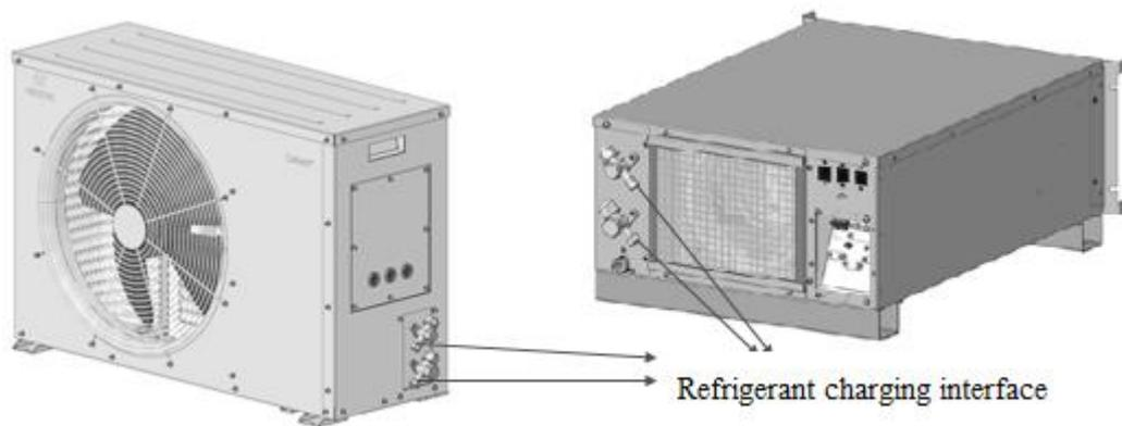
Figure 3-16 Refrigerant charging interface
