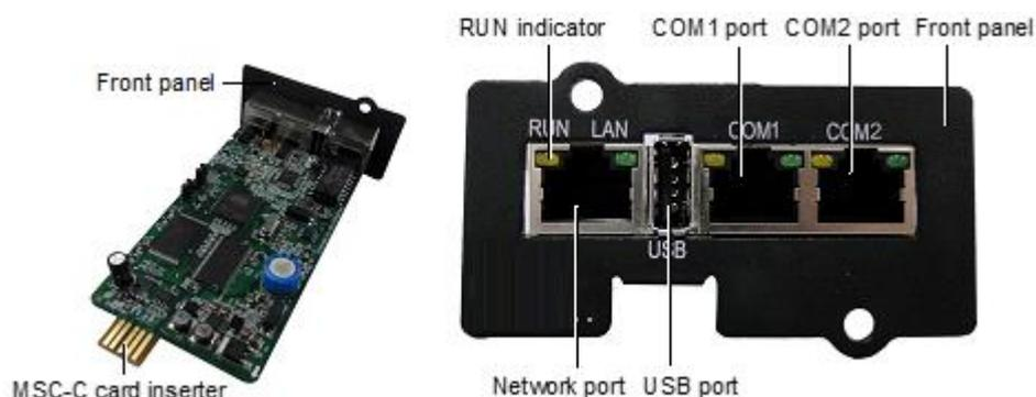
Figure 3-21 Appearance of the MSC intelligent monitoring card
