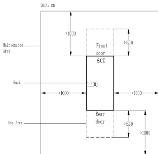
Figure 1-6 Space requirement of 600mm wide standard unit
