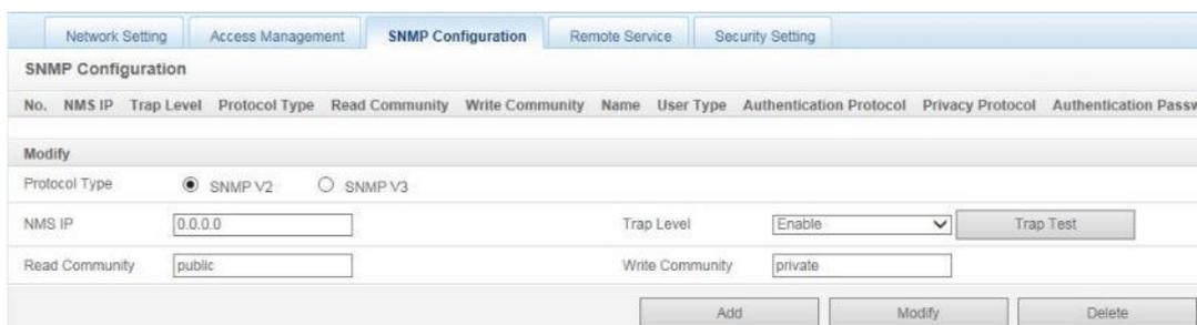
Figure 6-66 SNMP V2 setting
