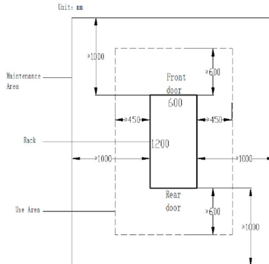
Figure 1-8 Space requirement of 600mm wide integrated unit
