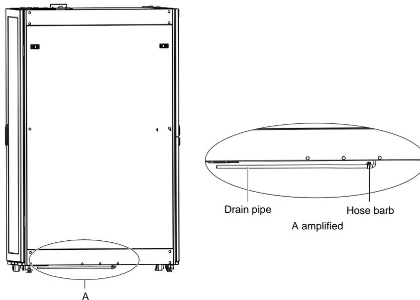
Figure 3-17 Condensate water pipe location
