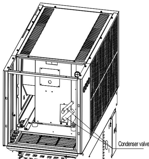
Figure 3-15 Operating drawing for opening the condenser valve
