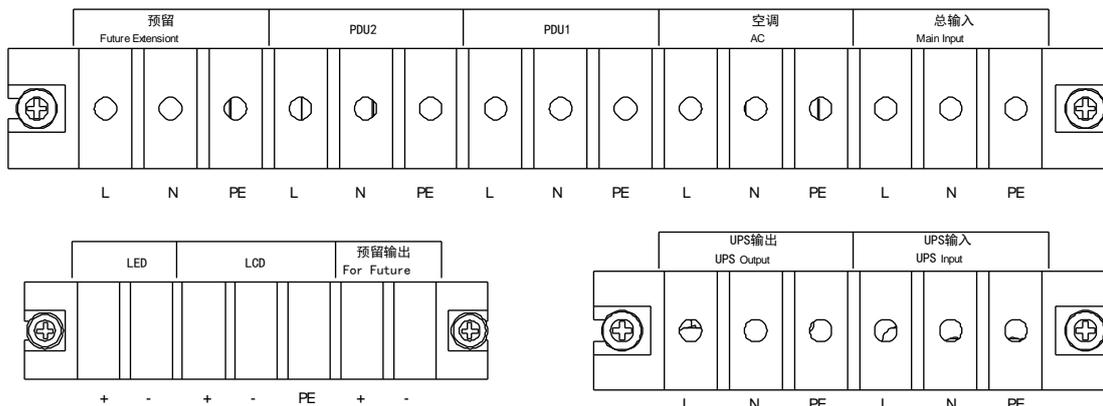
Figure 2 Silk printings of the PMU terminal block
