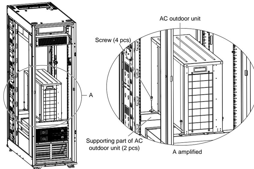
Figure 3-4 Removing the fixing screws of outdoor unit
