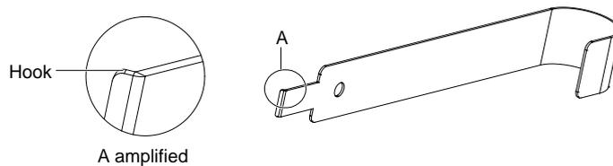
Figure 2-1 Floating nut hook
