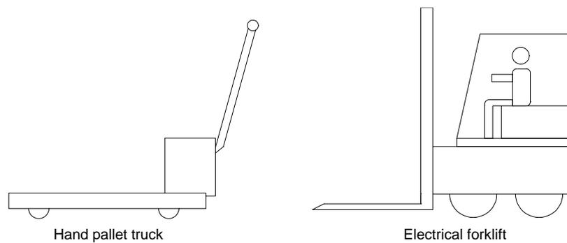
Figure 2-5 Mechanical carrying tools
