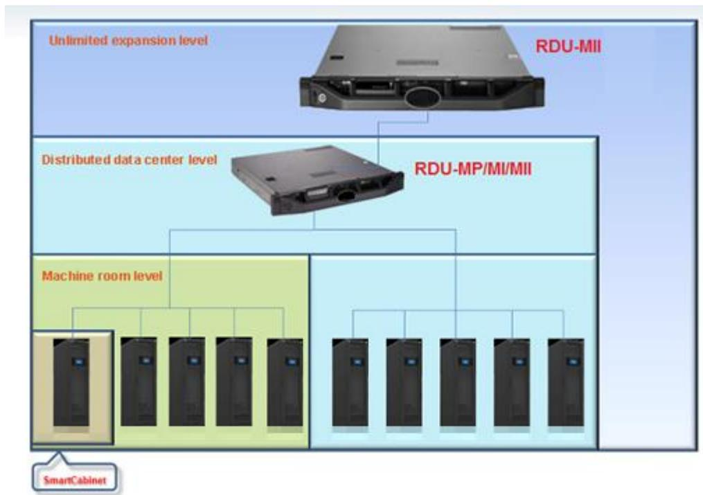
Figure 7-3 SmartCabinet networking topology diagram
