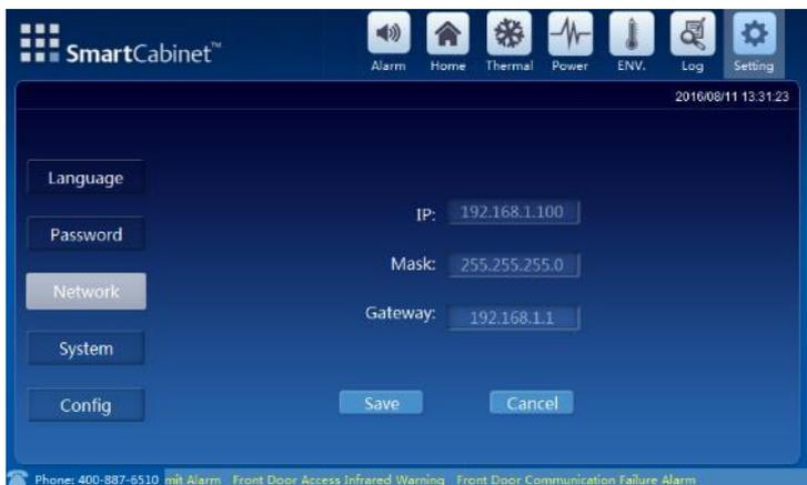
Figure 5-19 IP address setting screen
