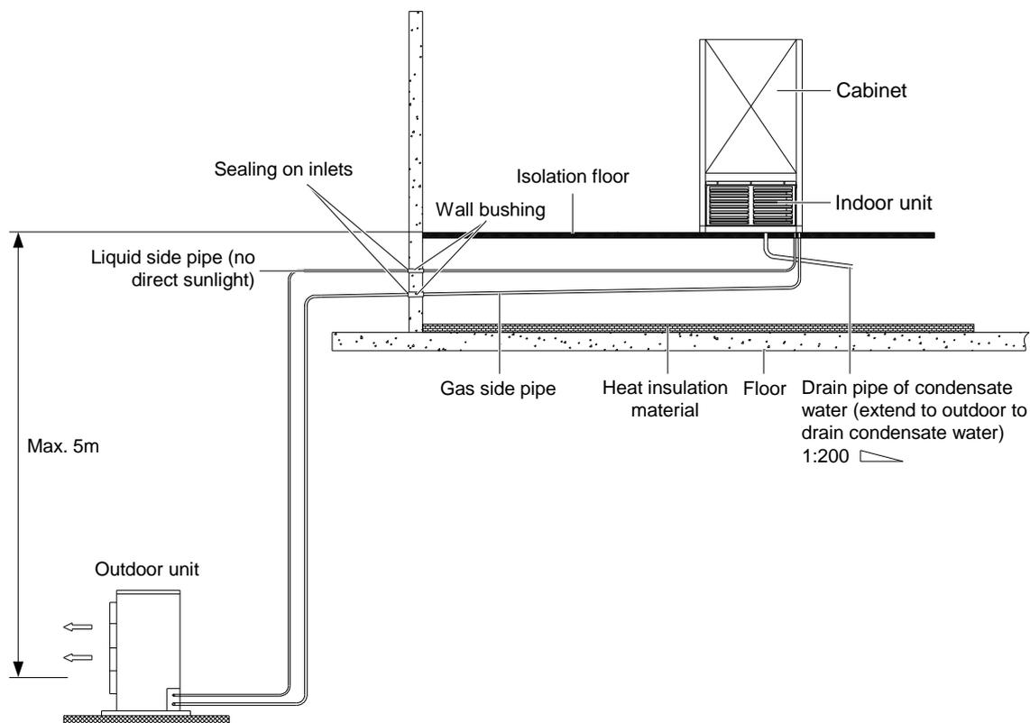
Figure 3-6 Outdoor unit installed lower than indoor unit
