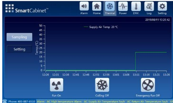
Figure 5-3 Thermal management acquisition data screen
