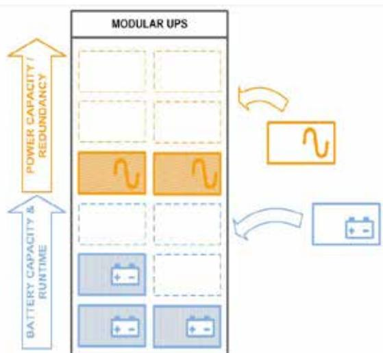
Figure 1: Modularity on power capacity or runtime.
