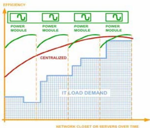
**Figure 3:** Efficiency in a modular versus a centralized UPS system
