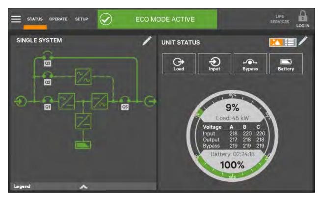
Figure 5.7 UNIT STATUS panel—Input details; graphic display
