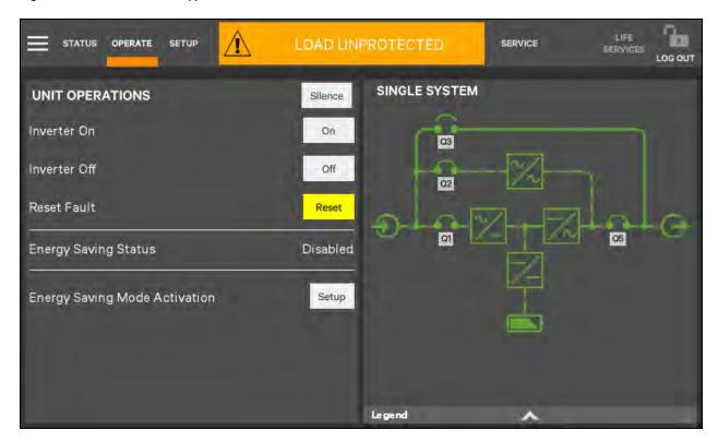
NOTE: In bypass mode, the load is directly fed by the mains power instead of the pure AC power from the inverter.
