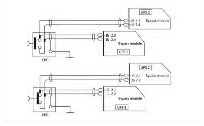
NOTE: In Figure 8.4 above, the upper one is Normally Open type, and the lower one is Normally Closed type.
