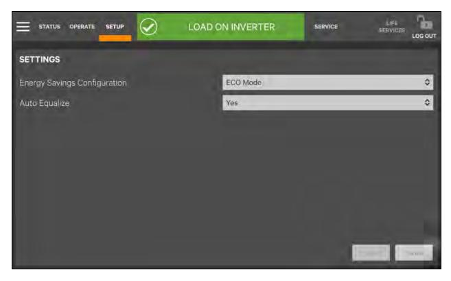
4. When the rectifier start process is finished, start the system according to Startup Procedures in Normal Mode. After the inverter runs normally, if the bypass voltage is within the range of ECO power supply, then the system works in ECO mode; otherwise the system will transfer to inverter. The system will automatically work in ECO mode after the bypass voltage is within the range of ECO power supply and lasts for five minutes.
