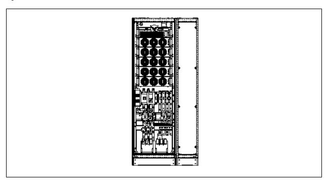
NOTE: When installing the two cabinets, remove the right-side panel of the main power cabinet first, and install the dismantled right-side panel on the right-side of the top cabling cabinet after the top cabling cabinet is installed.
