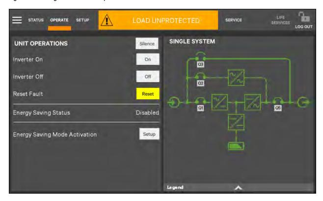
5. The inverter starts self-test and sync.
