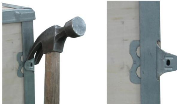
Figure 2-4 Straightening the hook
