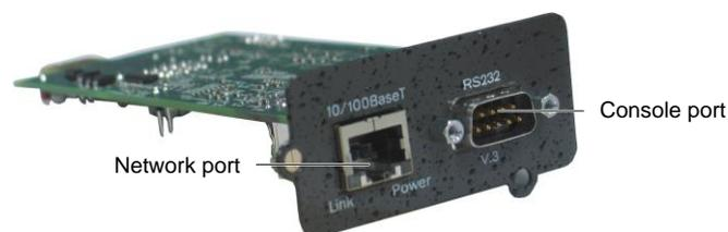
Figure 6-1 TCP/IP communication card
