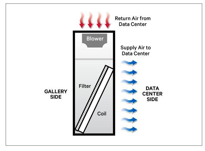
Figure 1.1 Downflow, horizontal-discharge blower configurations with EC fans
