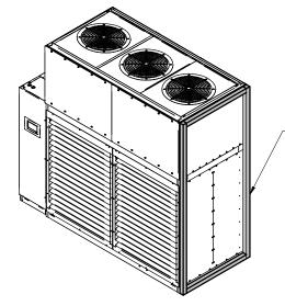
Gasketing shown is for pictorial purposes only to show edges of unit that require gap sealing. Gasketing and method to be provided and applied by others in the field.
