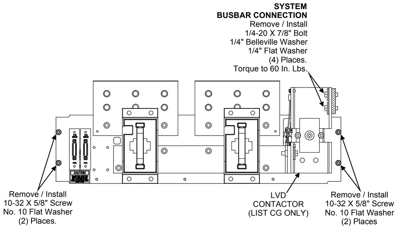
**Figure 26:** (Detail J) Replacing List NC
