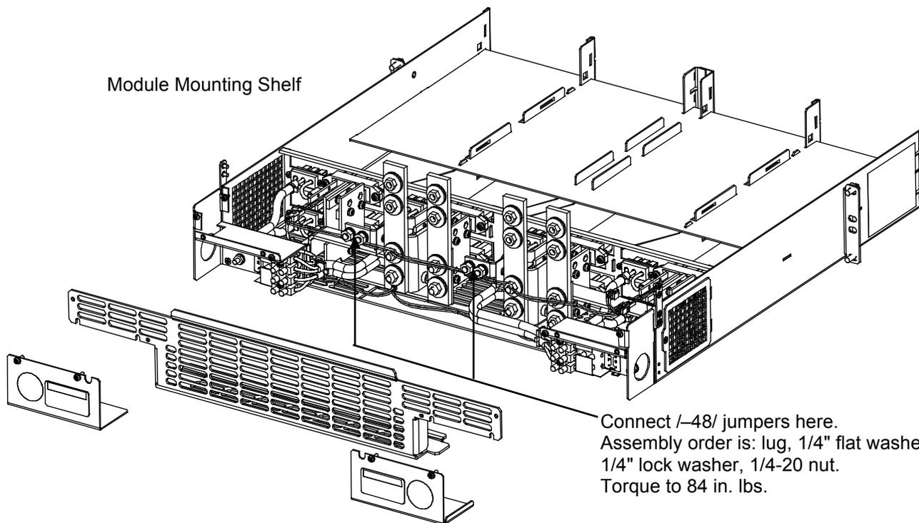
Connect /-48/ jumpers here. Assembly order is: lug, 1/4" flat washer, 1/4" lock washer, 1/4-20 nut. Torque to 84 in. lbs.
