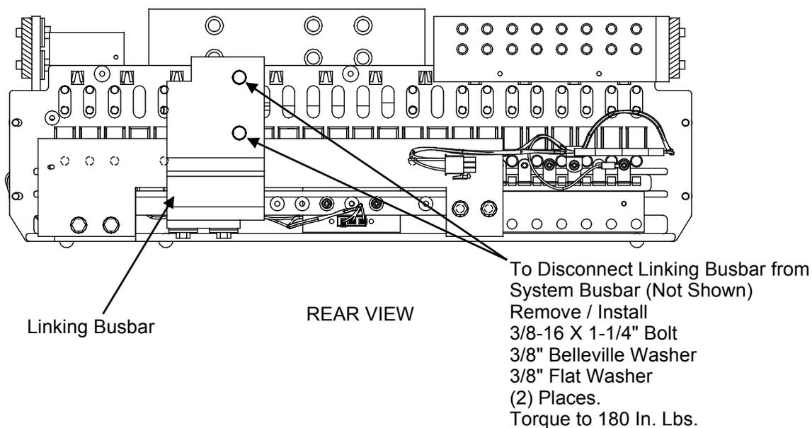
**Figure 26:** (Detail M) Replacing List AK
