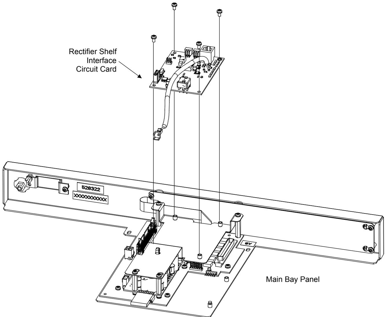
**Figure 14:** Replacing the Rectifier Shelf Interface Circuit Card in the Supplemental Bay Panel
