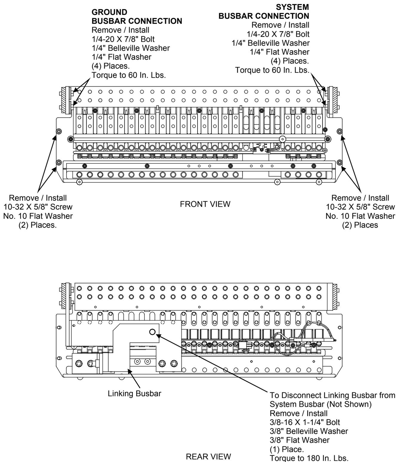
**Figure 26:** (Detail C) Replacing List NA
