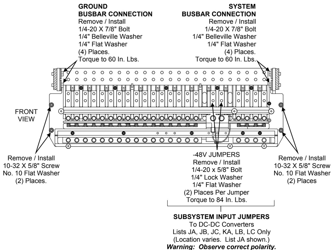
**Figure 26:** (Detail B) Replacing List EA
