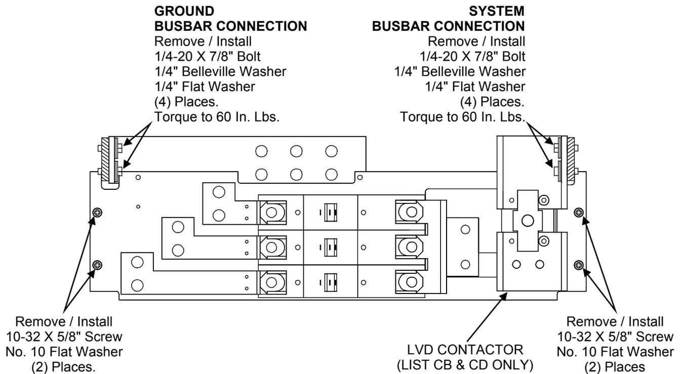
**Figure 26:** (Detail F) Replacing List CE (Lists AD, AE, and CF Similar)
