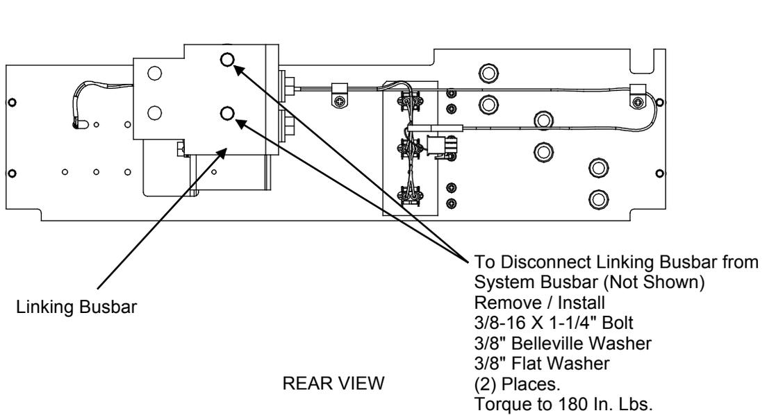
**Figure 26:** (Detail H) Replacing List CG (List AG, AJ, and CJ Similar)
