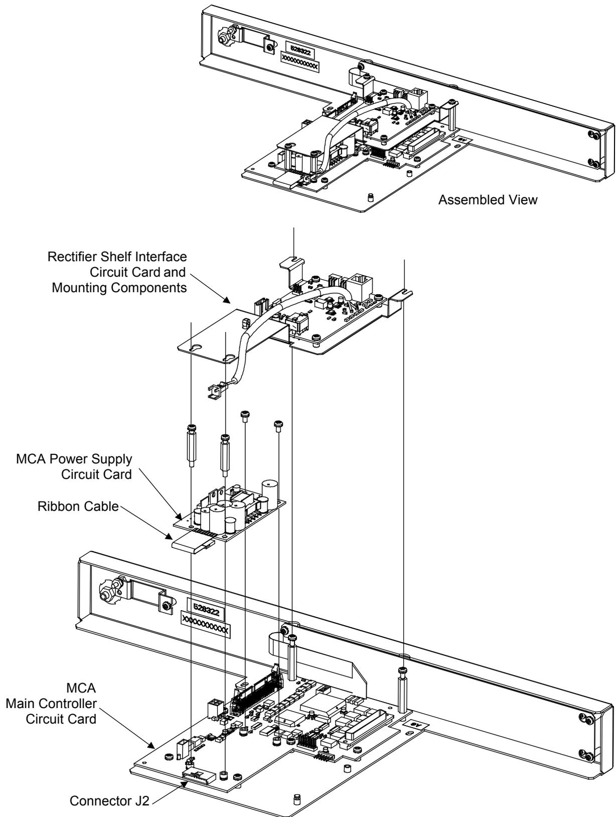
**Figure 11:** Replacing the MCA Main Controller Circuit Card
