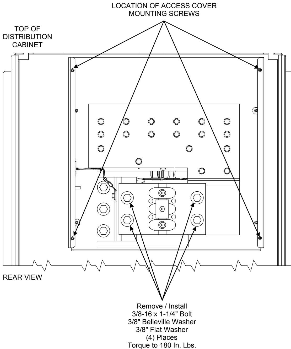
**Figure 29:** List RC Contactor Replacement Details (List RD and RE Similar)
