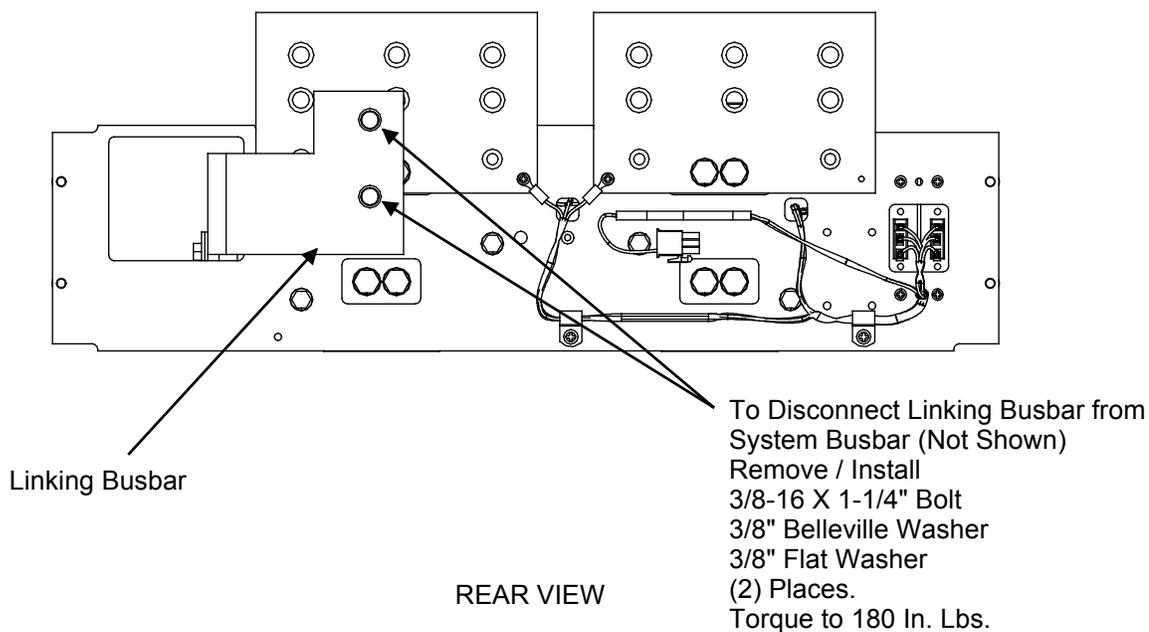
**Figure 26:** (Detail L) Replacing List GB
