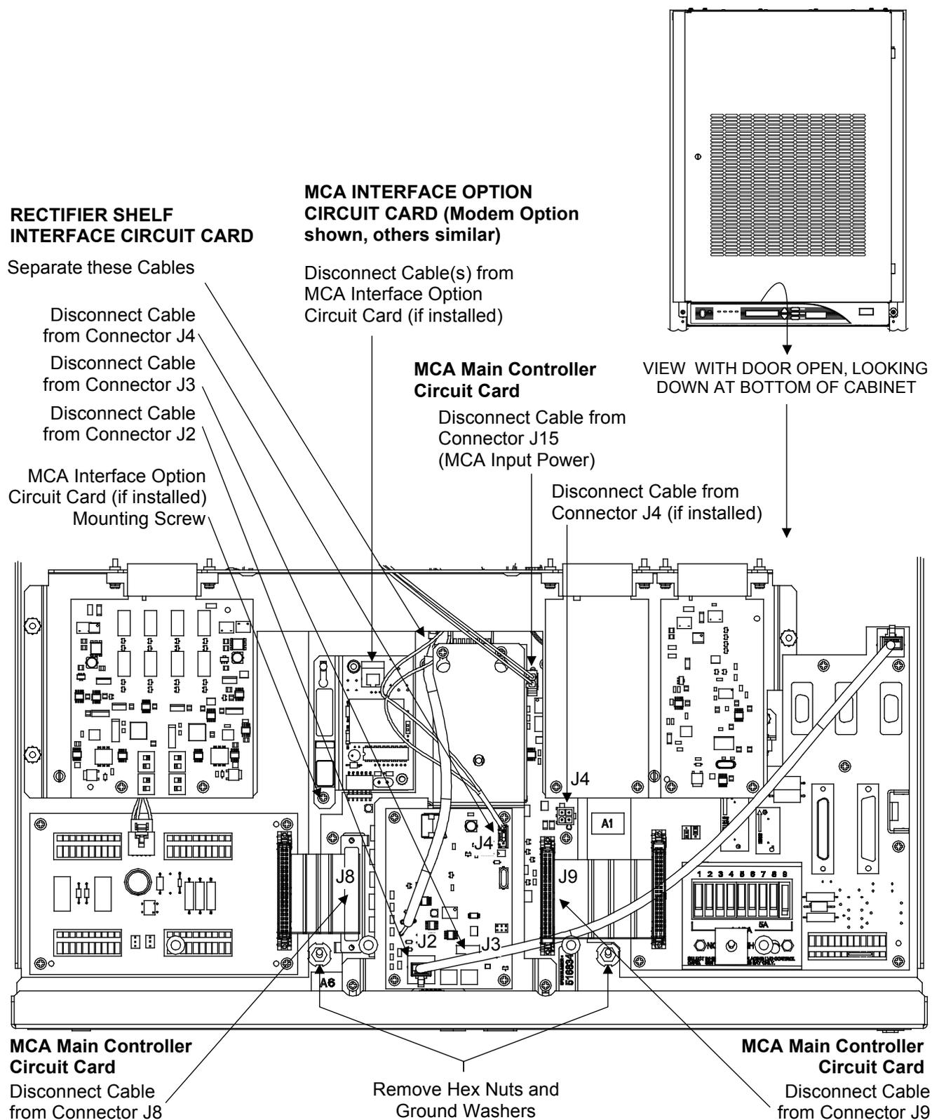
**Figure 10:** Replacing MCA Power Supply Circuit Card
