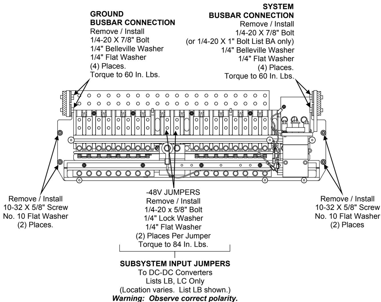
**Figure 26:** (Detail E) Replacing List CB (Lists AB, AC, and CD Similar)
