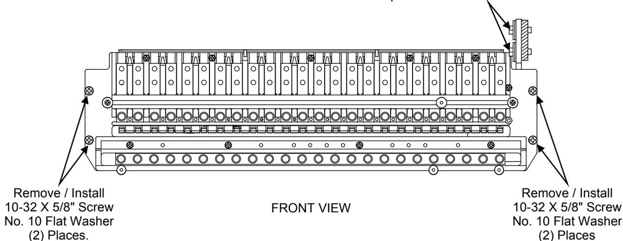
**Figure 26** (Detail N) Replacing List AL
