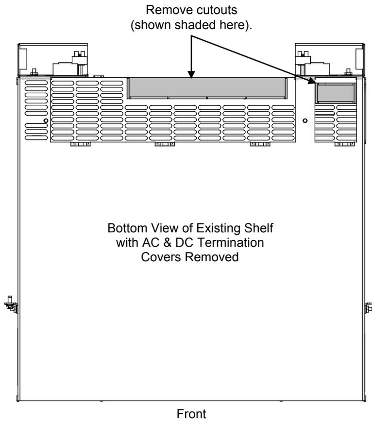
**Figure 5:** Installing Output Busbar Links Between Existing Shelf and Add-On Shelf
