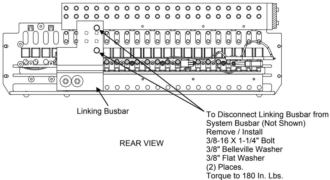
**Figure 26:** (Detail D) Replacing List LB (List BA, CA, and LC Similar)
