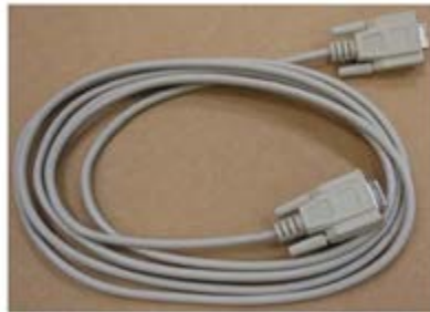
Figure 29 - RS-232 9 Pin Female to Female Cable
