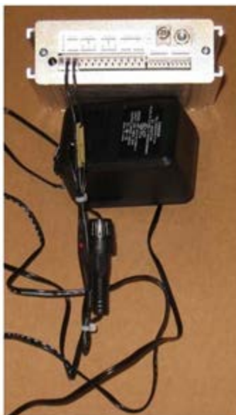
Figure 22 - Multitel's Float Charging Current Probe with Power Source and Inline Fuseholder
