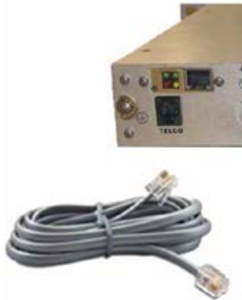
Figure 28 - TELCO RJ-11 Modem Connection
