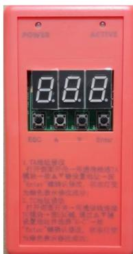
Figure 3-7 Modifying module address
