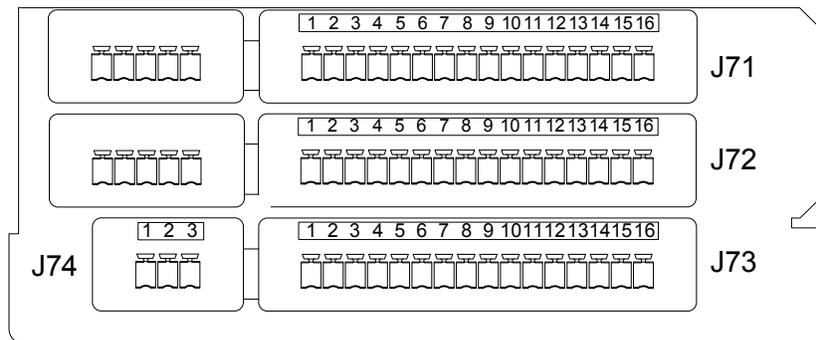
1. Customer control wiring connection points are terminals 1 through 15. (Pin 16 not used on J71, J72, and J73.)
