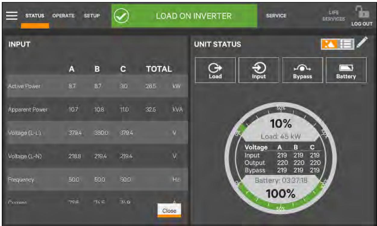
Figure 5.8 UNIT STATUS panel—Bypass details; graphic display
