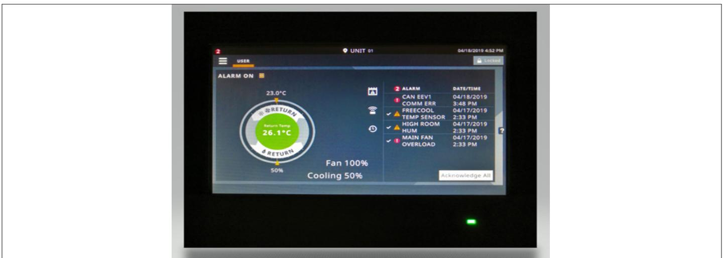
**Figure 1-3 iCOM Controller Display**
