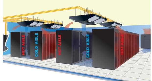
The Liebert XDO systems work extremely well with the "hot aisle-cold aisle" approach.
