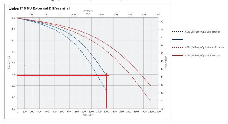
1368 kW heat transfer at 7.2°F (4.0°C) ATD - facility water at 89.6°F (32°C) W3
