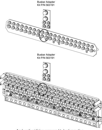
Apply anti-oxidizing compound to busbar mating surfaces before assembling.
