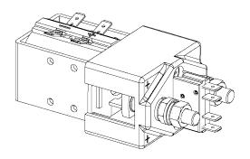
The load contactor(s) are wired with a pigtail jumper harness that plugs into a mating connector located in the power system wire harness.
