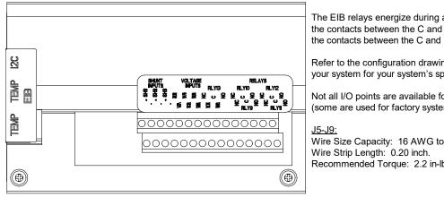
The EIB relays energize during an alarm condition, closing the contacts between the C and NO terminals, and opening the contacts between the C and NC terminals.
