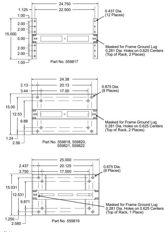
Figure 4.1 Relay Rack Floor Mounting Dimensions - 23" (cont'd from previous page)
