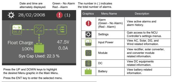
To reboot the Controller, from the Main Menu press the ENT and ESC keys at the same time. Release both keys. Press ENT to confirm.
