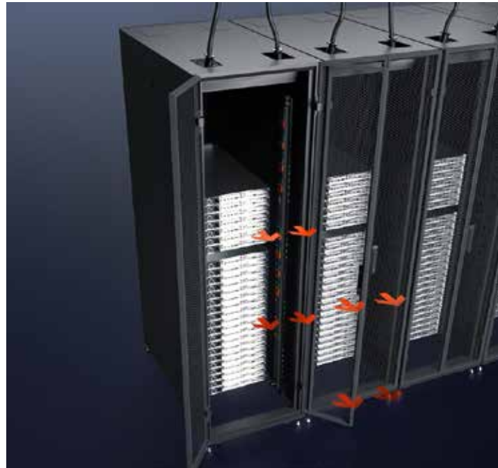
Standard CPU Hot air from server fans
