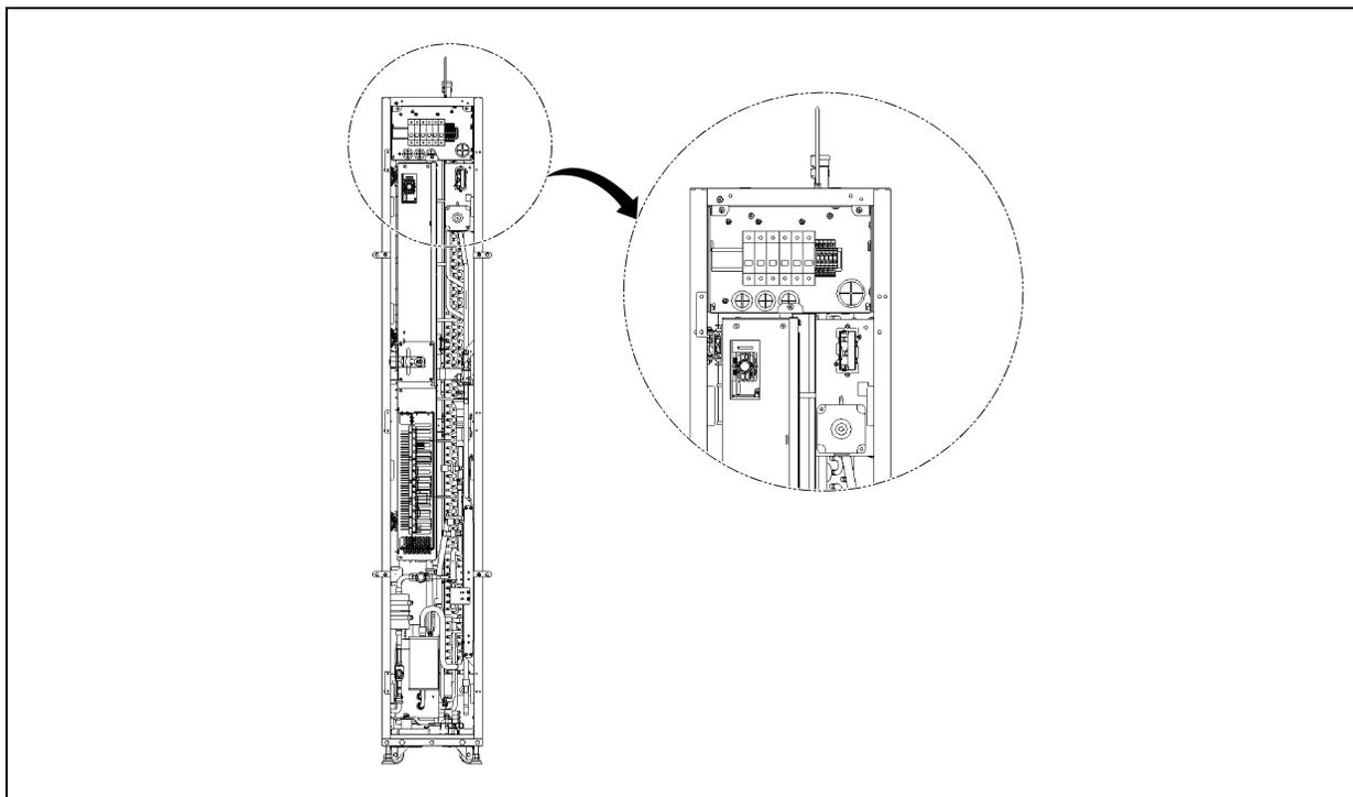
**Figure 5.2 Electrical Control Box (Three Phase Unit)**
