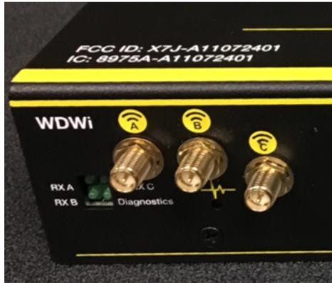
Once the antennas are secure, you'll need to ensure proper antenna position. Antennas A and B can be close together, but to avoid signal interference they both need to be as far away from antenna C as possible. Extend the leader cables on the antennas to their fullest lengths and secure the antennas as far away from the Watchdog Wi, and as high off the ground as possible.
