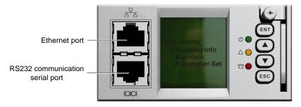
Figure 2-20 M221S controller communication port
